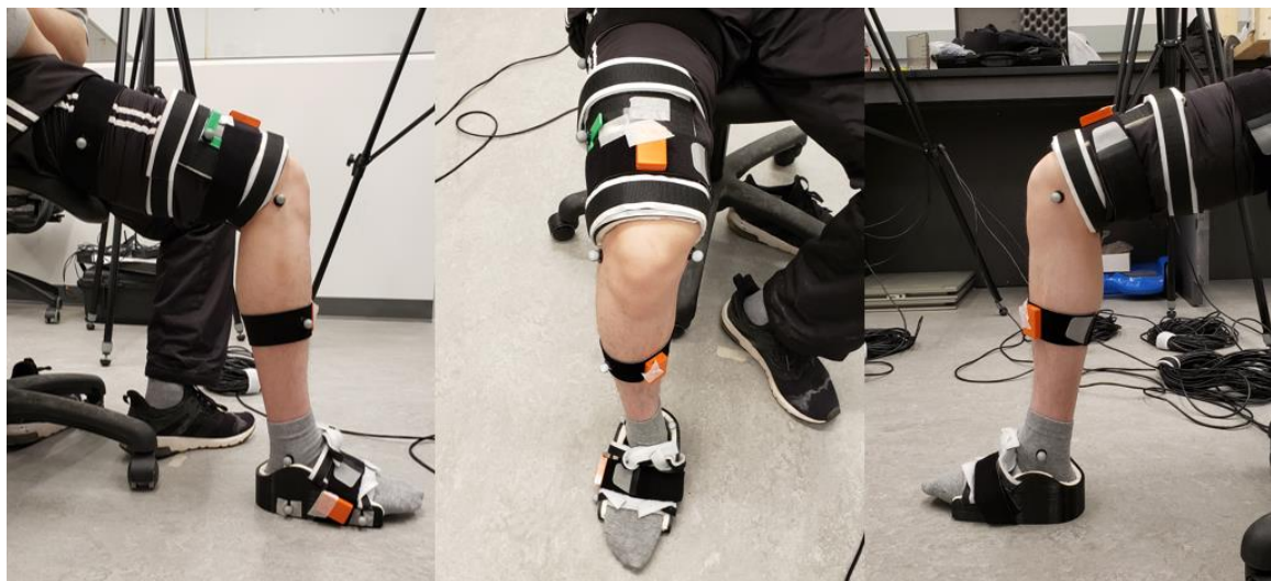
Figure 16. Validation setup for Xsens IMUs and algorithms against VICON motion capture
