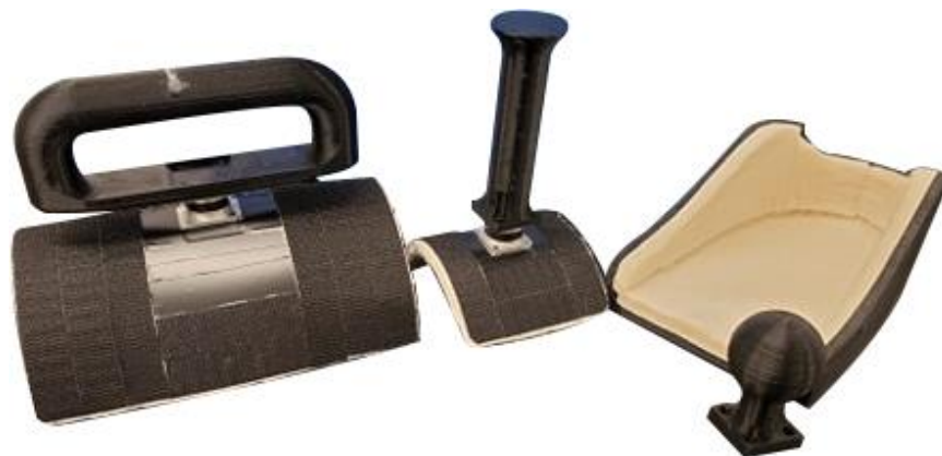
Figure 9. Experimental setup for (left to right) thigh, shank and foot. The spherical handle is attached to the bottom of the foot brace.
