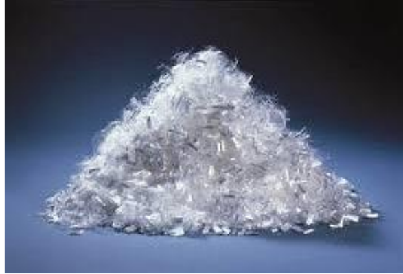
Figure 2-5: Polypropylene fibres (Wafa, 2018).
