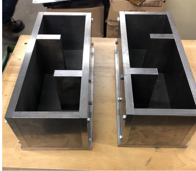
Figure 2-7: Shear mold for double shear test.
