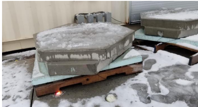
Figure 3-8: Concrete paver fabricated in Sidewalk Lab Toronto [Photograph taken: Jan. 2020].
