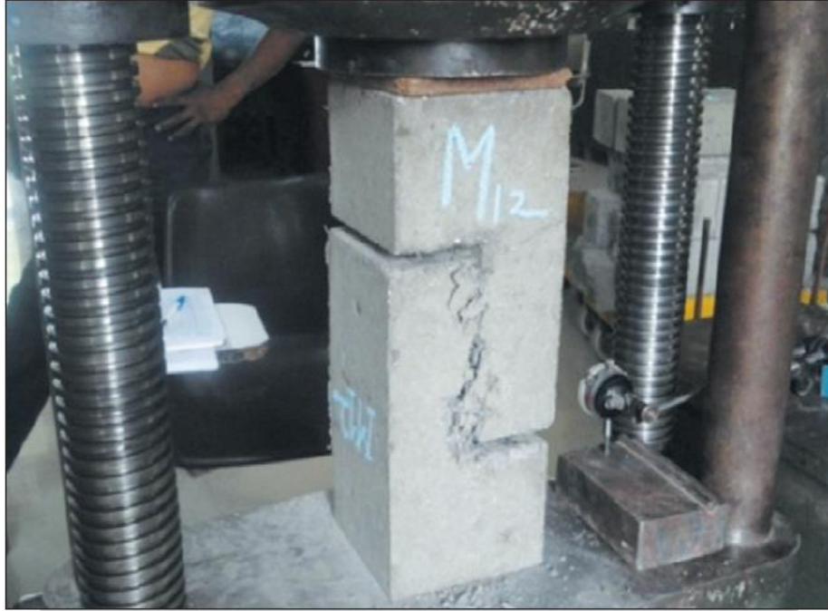
Figure 2-8: Specimen under the double shear test (Kalwane, 2016).
