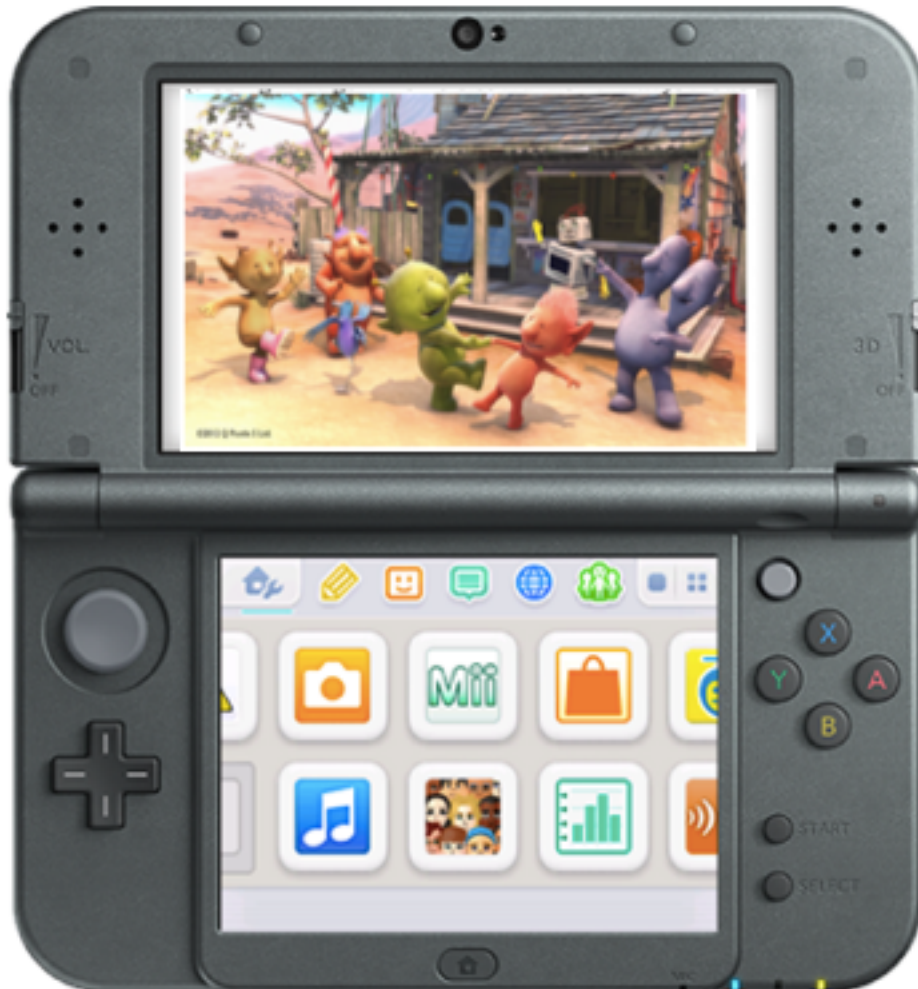
Figure 12. An example of the Nintendo 3DS system. The movie is displayed in the upper screen while the bottom touch screen can be used to control the device.
