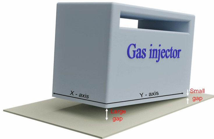
Figure 10.4. Schematic representation of a tilted AP-CVD reactor head placed above a substrate. By adjusting the reactor-substrate spacing along the length of the head, a film thickness gradient can be obtained.
