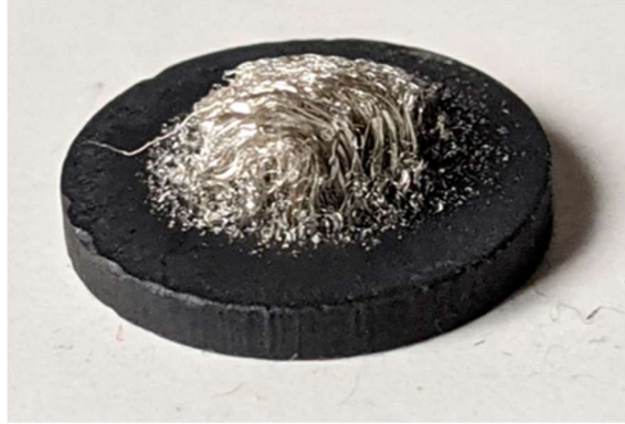
Figure 5.9. Pellet of ‘Ag 8.1 SnS 6 ’ after the thermal diffusivity measurement up to 785 K.
