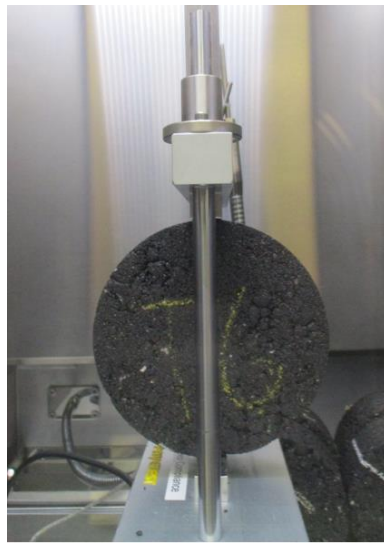
Figure 3.7 IDEAL-CT Test Loading Fixture.
