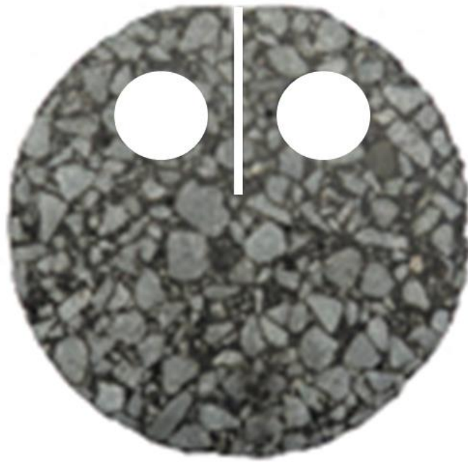
Figure1. DC(T) specimen (A full disc including an edge cut, a notch and two loading holes)
