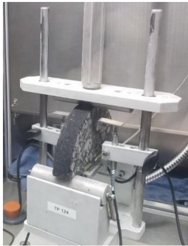
Figure 3.5 SCB Test Loading Fixture.
