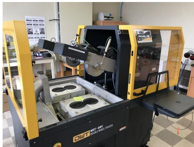
Figure 3.11 Hamburg wheel tracking device.
