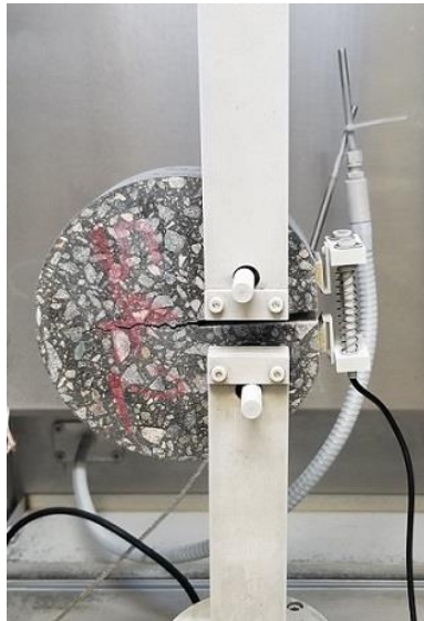
Figure 3.3 DC(T) Test Loading Fixture.
