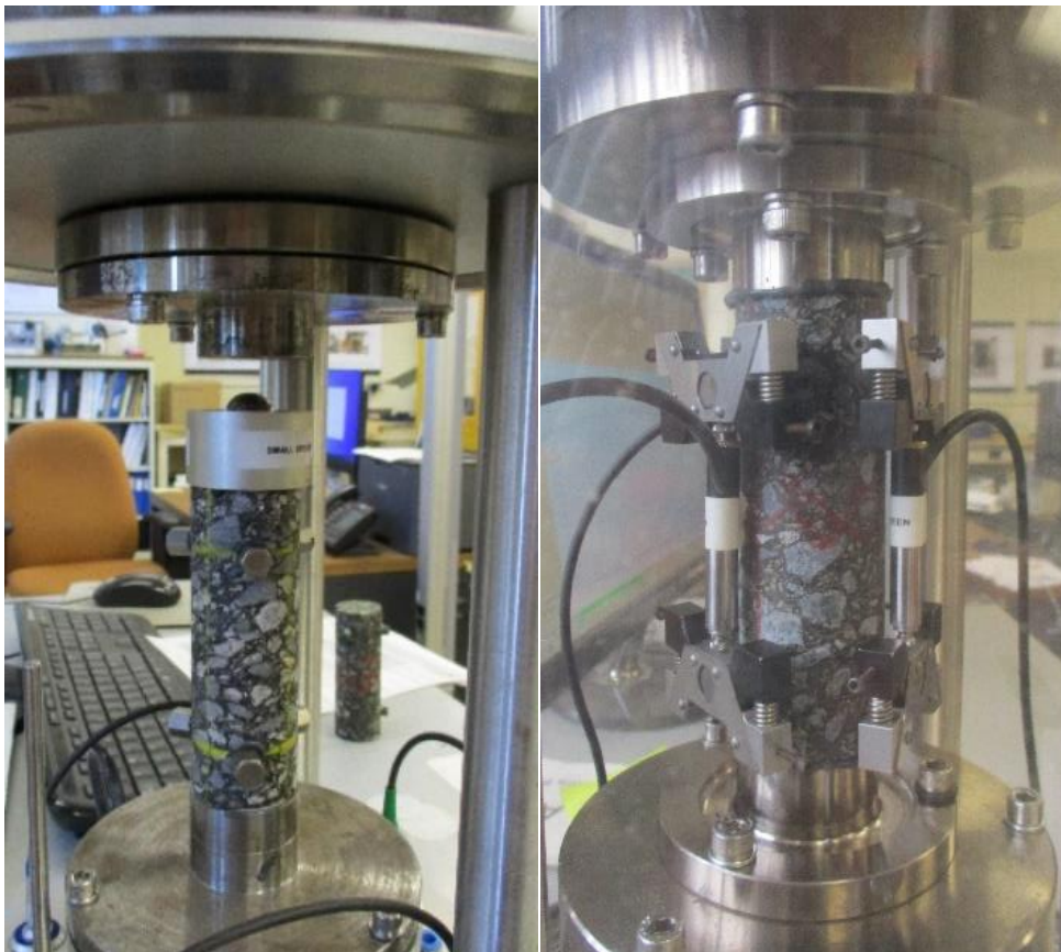
Figure 3.10 Complex Modulus Test ( left ) and Cyclic Test ( right ).
