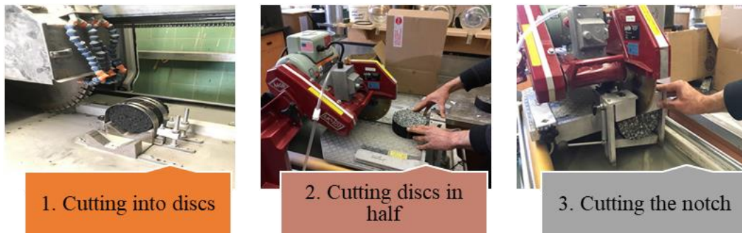
Figure 3.9 The procedure of I-FIT Specimen Preparation.
