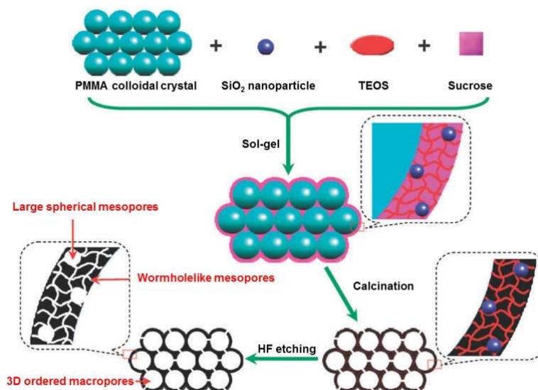
Figure 2.5 Synthesis of hierarchical porous carbons via a ternary-nanocasting strategy. 67
