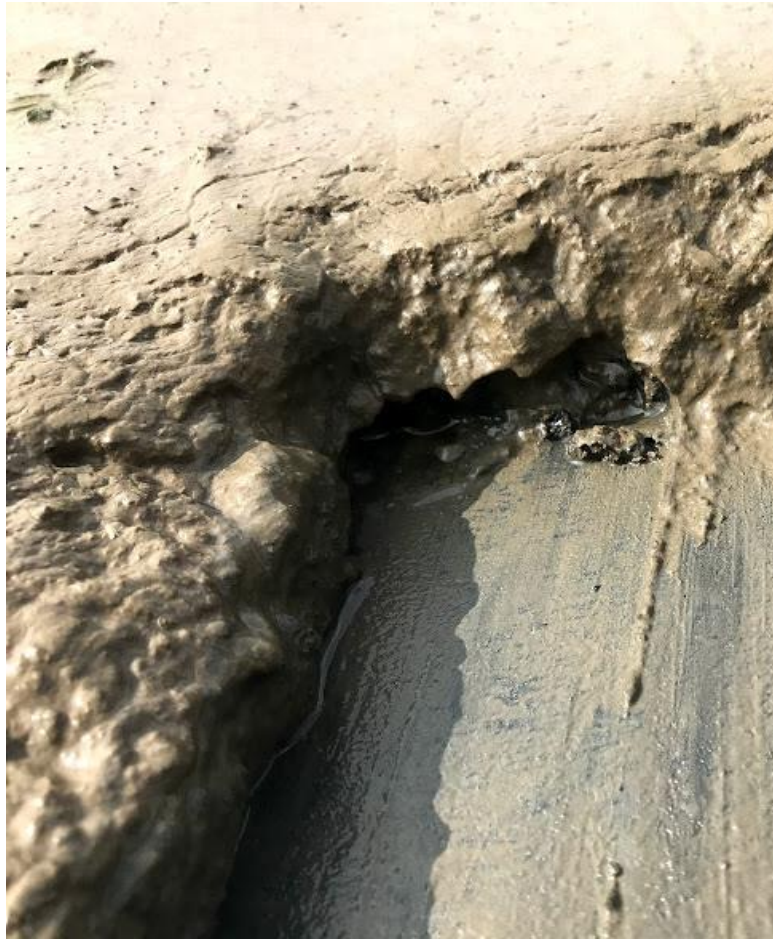
Figure 3-3: Deposited sediment collected from HVR Cell#1 in September 2020. Two distinct layers are evident: (1) a thin top layer of loosely bound fine sediment that deposits at low flow (sometimes referred to as surficial fine-grained laminae (Droppo & Stone, 1994) and (2) a more consolidated bottom layer. The cell was dredged in October 2019. Approximately 3 to 4 inches of sediment deposited in the cell during the subsequent year.
