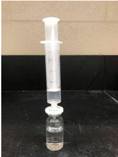
Figure G5: Dredging efficacy experiment process. A) add water to centrifuge tube spiked with various phosphate concentrations and agitate for 18 hours on shaker table, B) if coagulant is to be added, after 18 hours of agitation set centrifuge tubes upright and add range of coagulant dose and type, rapid swirl for 10 seconds, and C) filter sample through 0.45 \mu\text{m} filter before analyzing final phosphorus concentration using ammonium molybdate/stannous chloride method
