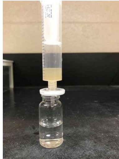
Figure G4: Sorption experiment process with coagulant amendment. Steps A) and B) the same as figure G3-A and G3-B, III) after 18 hours of agitation, set centrifuge tubes upright and add range of coagulant dose and type, rapid swirl for 10 seconds, and IV) filter sample through 0.45 \mu\text{m} filter, before analyzing final phosphorus concentration using ammonium molybdate/stannous chloride method
