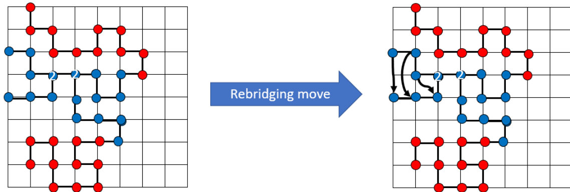
Figure 2.4: Example of the polymer rebridging move. For simplicity, the move is demonstrated on a two-dimensional simple square lattice. The sites with two monomers on them are marked with the number 2.
