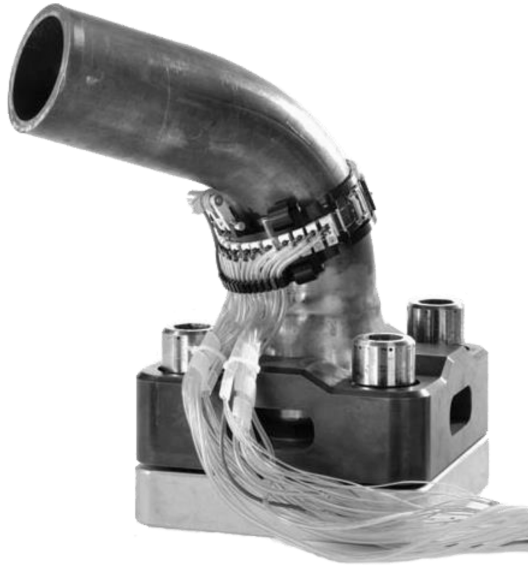
Figure 5.17: A typical bracelet type ultrasonic tool used for feeder pipe inspections. (Image courtesy of ZETEC ® , reproduced with permission.)
