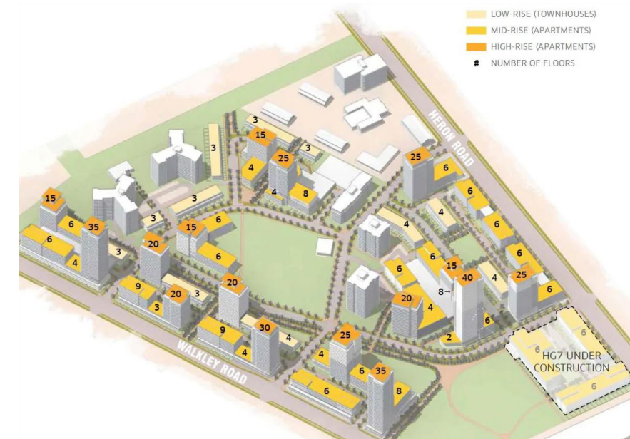
Figure 3.21 Heron Gate Redevelopment by Timbercreek - Massing diagram (Heron Gate Village Planning Rationale Report & Urban Design Study, 2019)
