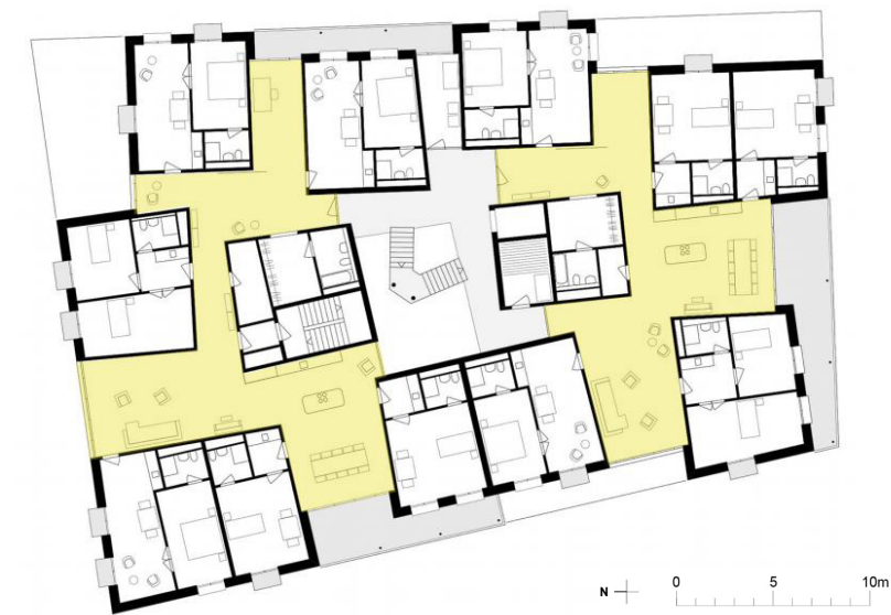
Fig. 4.9 The floorplan of House A by Duplex Architekten, showing a cluster house building that draws from the planning strategies of the development and implements a similar pattern of built form and connective spaces within the building itself. The social shared spaces highlighted in yellow to illustrate the private-public relationship of the floor plan (Brysch, 2019).
