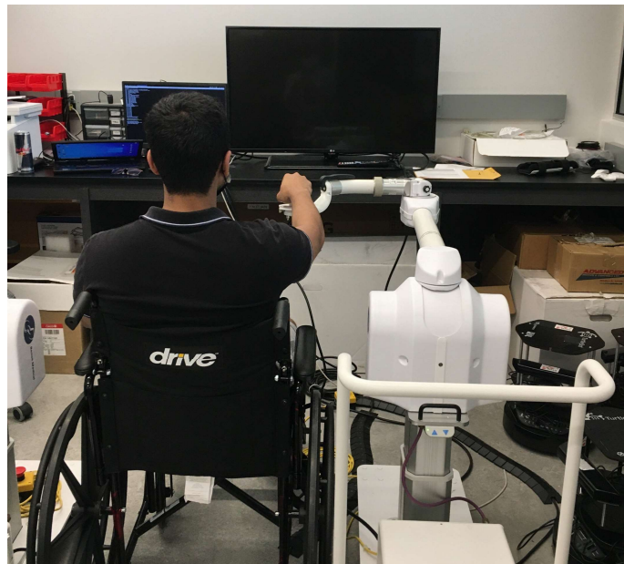
Figure 2.1: A user participating in an experiment on the Barrett Upper-extremities Robotic Trainer (BURT).
