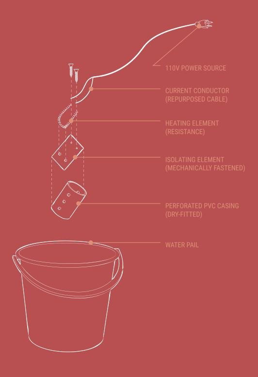
Fig 38. Water Heater Component Breakdown
