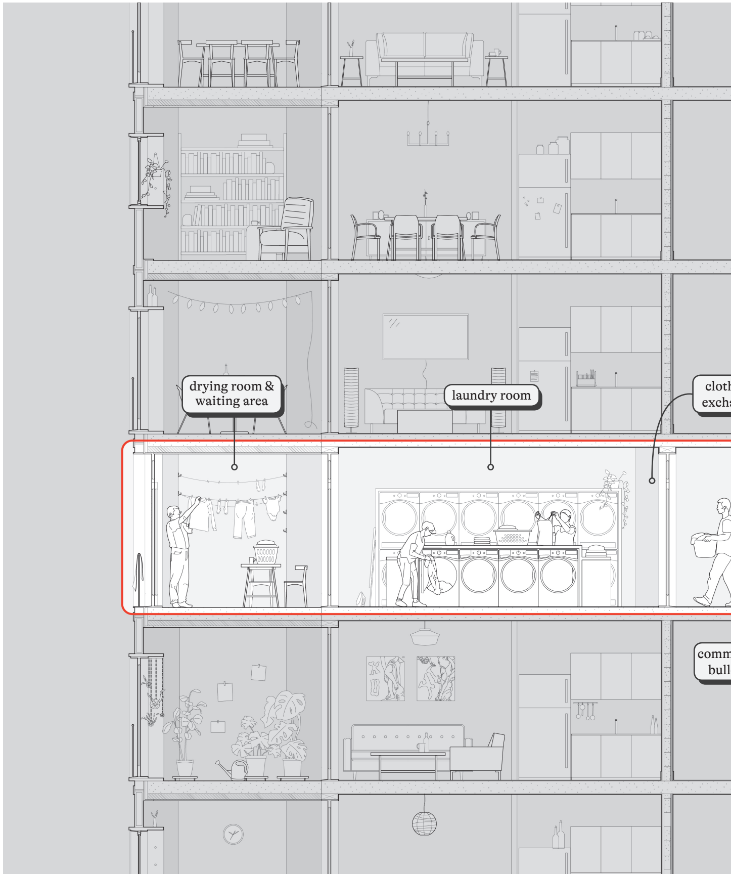
[fig 58] section through tower at new laundry room + hobby workshop communal space
