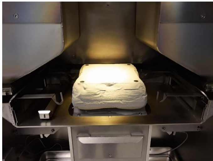
Figure 2.4 Figure depicts a completed build showing the sintered powder cake. This cake will be taken to the PRS to extract final parts.
