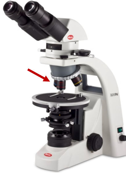
Figure 2.1: Motic Binocular microscope that is commonly used for examination of biological tissue specimen in histopathology. The red arrow points at objectives of the microscope for setting the magnification level.
