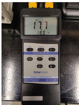
Figure 3.4 Fisherbrand thermocouple reader used to measure solution and ambient temperatures simultaneously.
