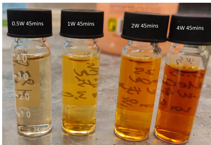
Figure 5.12 Solution color changes of femtosecond irradiated WS 2 with varying laser powers (0.5, 1, 2, 4W for 45 minutes).
