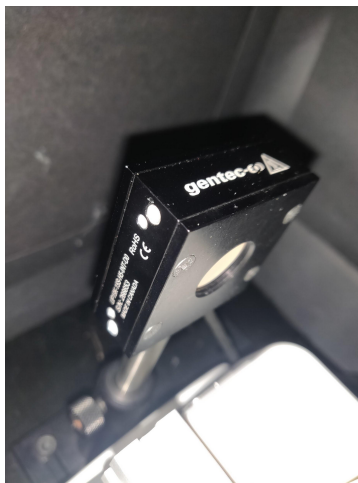
Figure 3.6 Gentec-EO laser power meter used to determine the power of the NIR laser.
