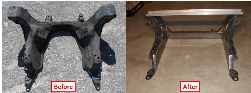
Figure 8: Stock [80] versus modified [81] cradle for Mazda Miata
