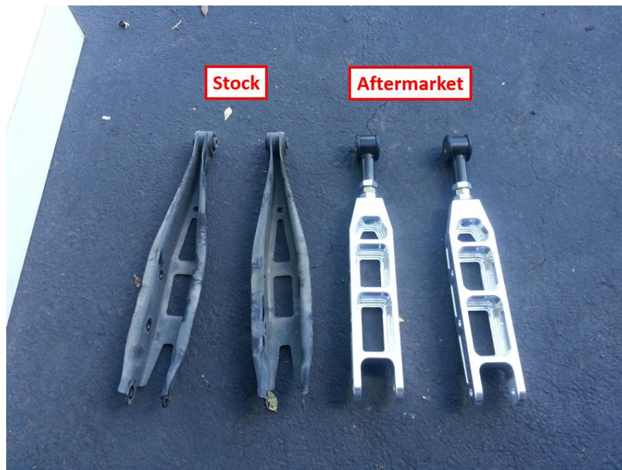
Figure 7: Example of stock and aftermarket control arms [79]
