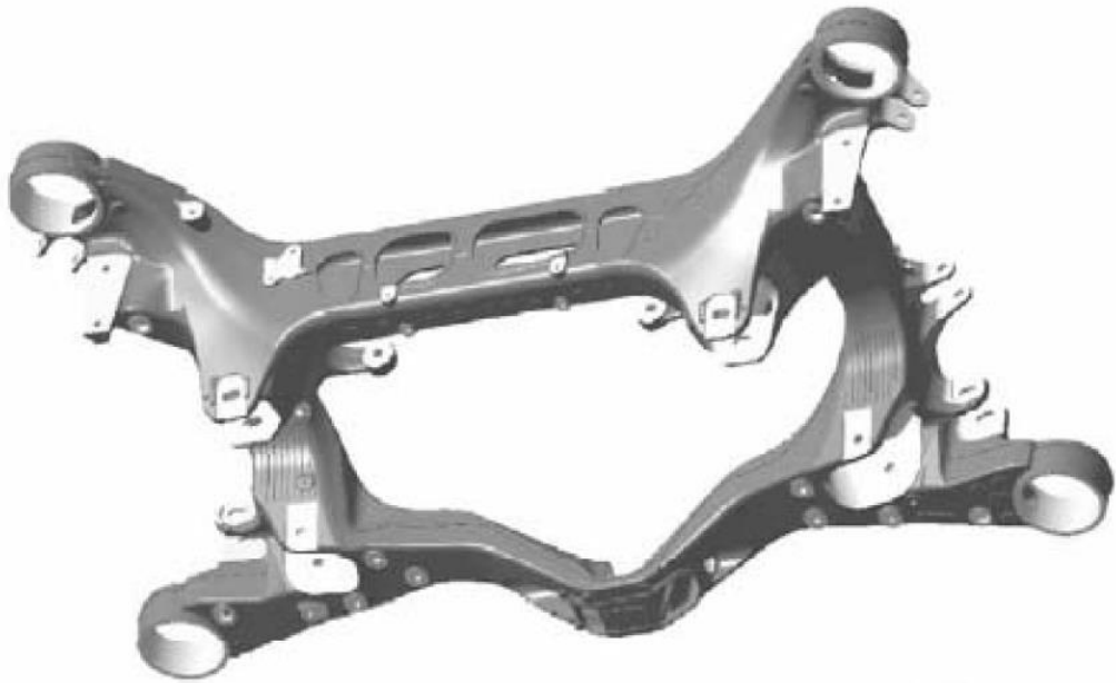
Figure 63: Die-cast aluminum cradle for Porsche Panamera [19]
