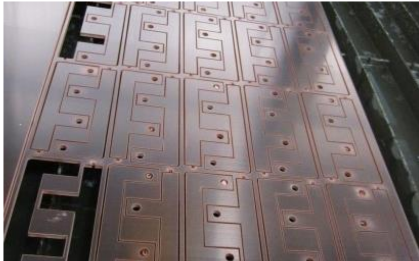
Figure 96: Example of waterjet nesting, showing close proximity of parts to minimize material waste [141]
