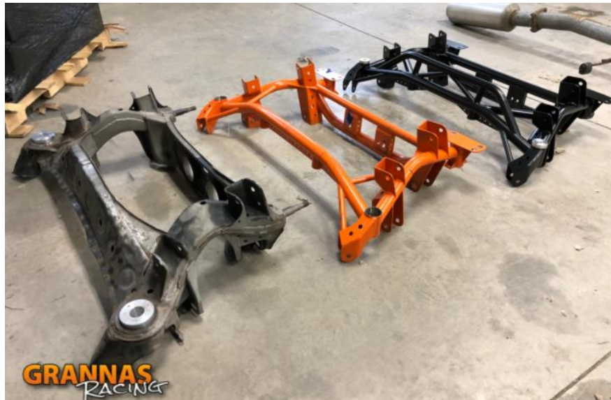
Figure 9: Stock (left) versus aftermarket cradles (right) for Toyota Supra [82]
