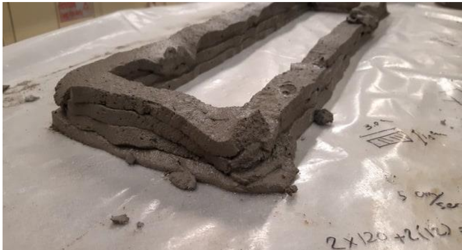
Figure 3-17, manually printed layers using WC0.39SP0.5
