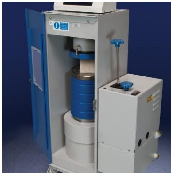
Figure 3-28, ELE International model #36-3088/02 concrete compression testing machine
