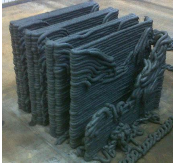
Figure2-30, Visual evaluation of Buildability Property (Le, et al., 2012)
