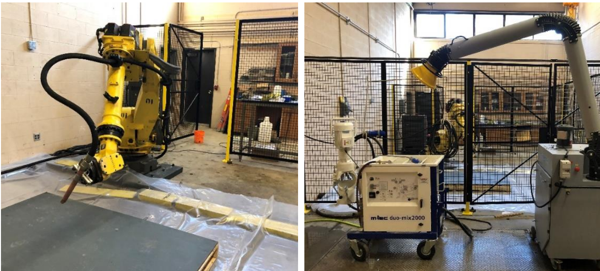
Figure 3-11, 3D-Printing lab at UW: a)- FANUC R- 2000iA/ 165F, b)- M-Tec duo-mix 2000
