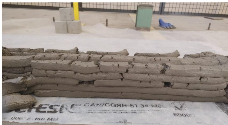
Figure 3-21, The printed layers by WC0.36SP0.19
