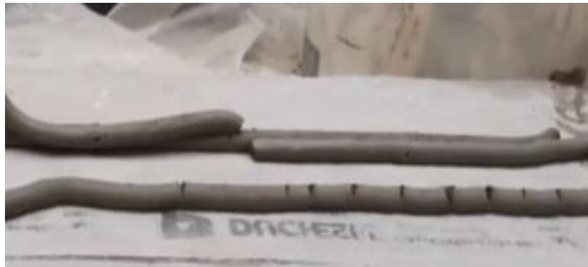
Figure 3-22, The printed layers by WC0.36SP0.3
