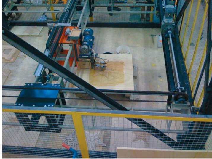
Figure2-9, Concrete printing technology (Jianchao, Zhang, Faried, & Wengang, 2017)
