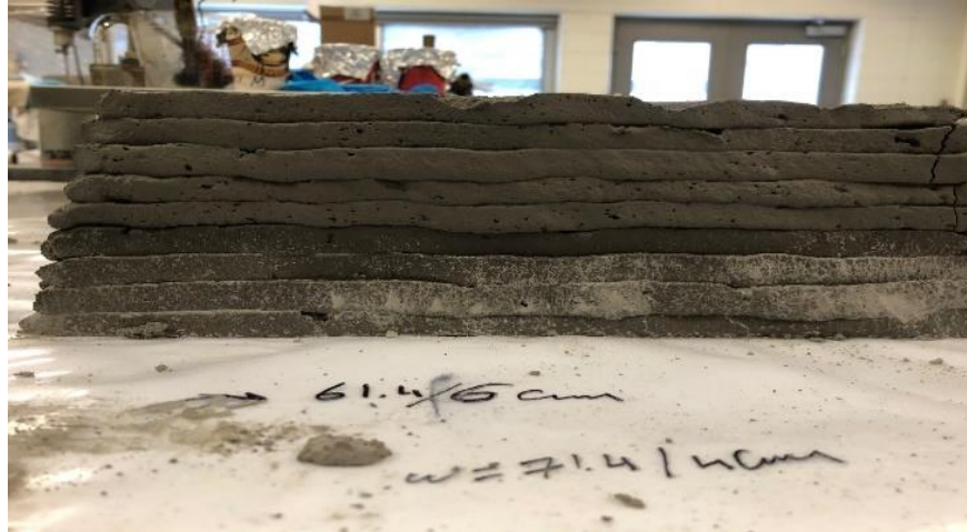
Figure 3-16, manually printed layers using WC0.39SP0.25
