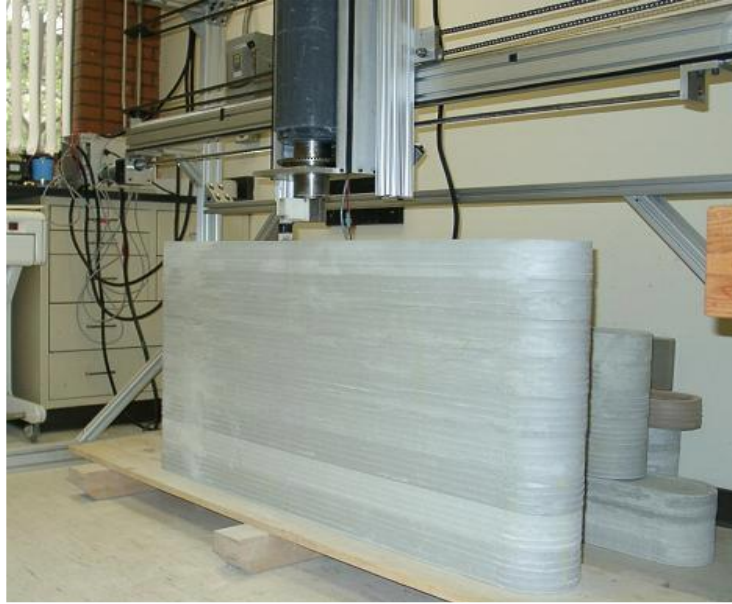
Figure2-4, 3D- printed concrete wall fabricated by CC machine (Khoshnevis, 2004)
