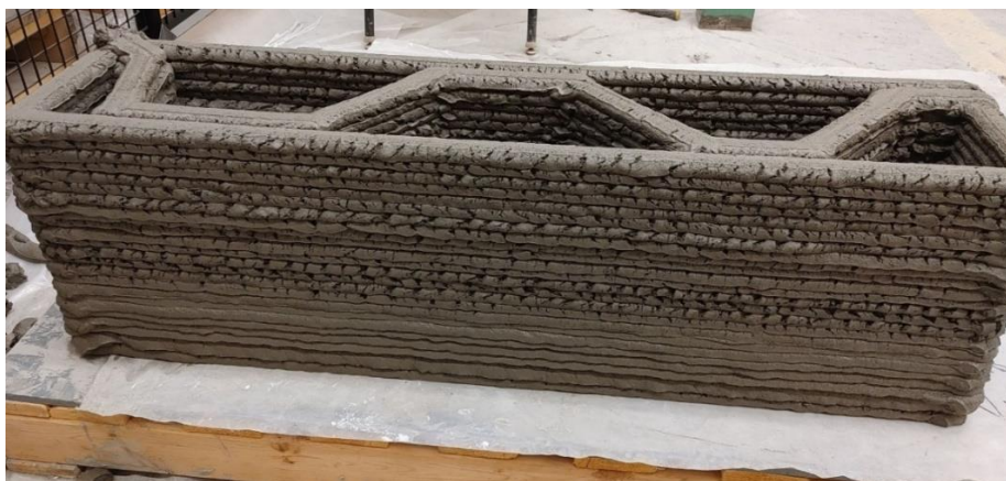
Figure 3-23, 3D-Printed wall (1010*235*315 mm) at UW
