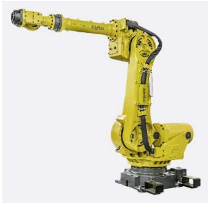
Figure 3-9, Research's robot arm (FANUC R- 2000iA/ 165F)
