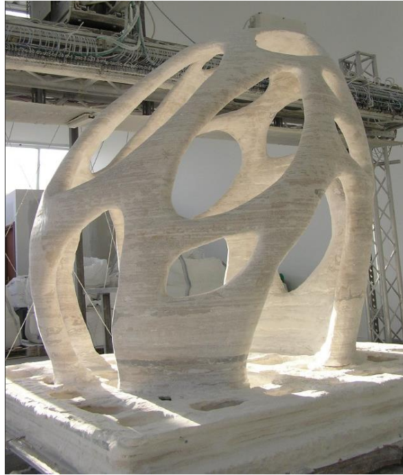
Figure2-8, Radiolaria pavilion fabricated by D-Shape technology (Dini, 2006)
