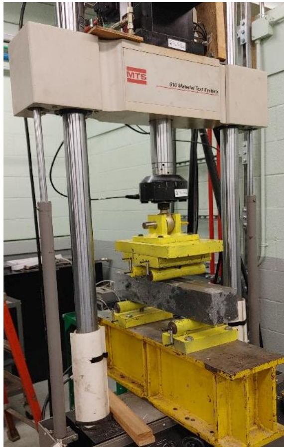
Figure 3-38, MTS machine for flexural testing
