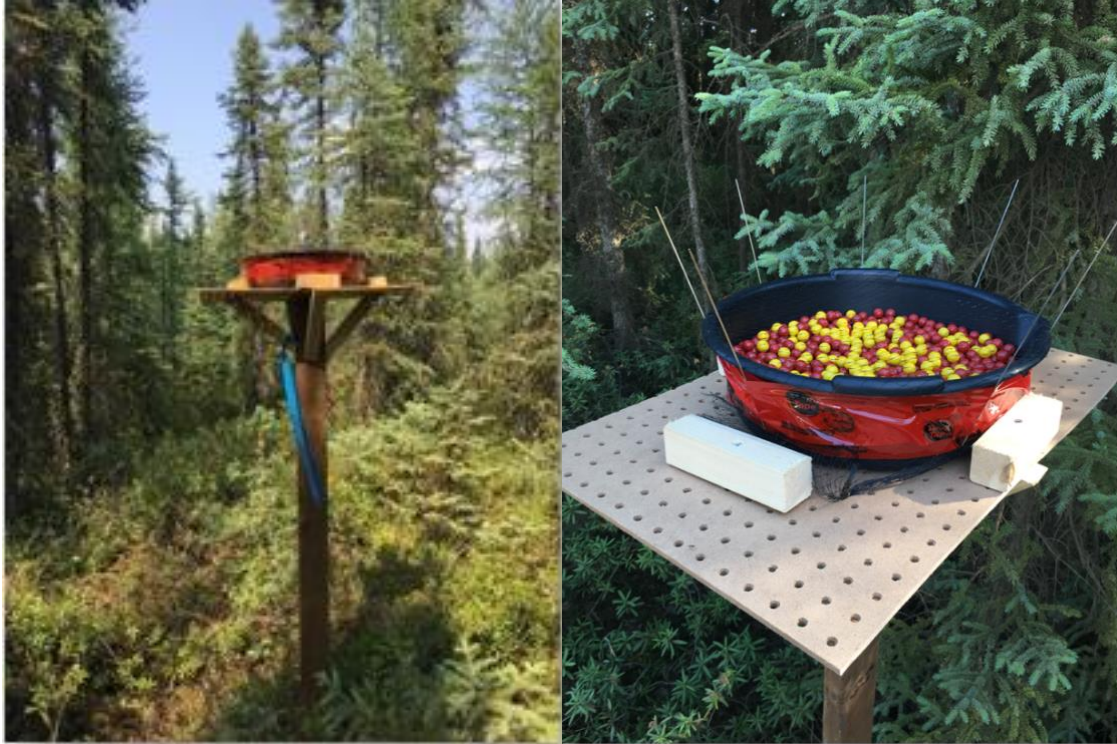
Figure 3-3. Images of atmospheric dust collectors used in August of 2019 to capture dust deposition from the nearby, unpaved road, Heaven Swamp, Fort McMurray, Alberta, Canada.
