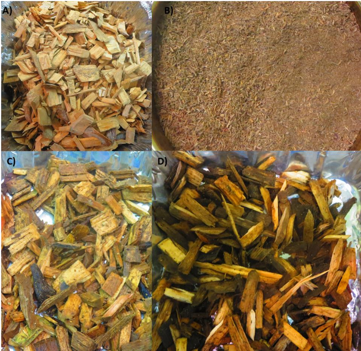
Figure 4.1 The Filtrexx® material before use (A), after being ground to <2\text{mm} (B), after use at ILD and after use at LON (D).
