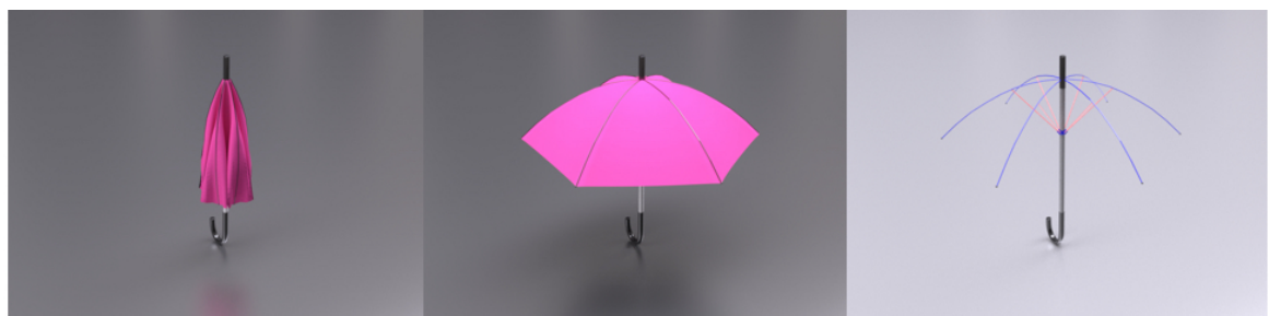
Figure 6.5: Umbrella: An umbrella closed, open, and shown with only the wireframe rod-edges rendered. The rod sub-component of the mesh contains non-manifold triple-junctions.
