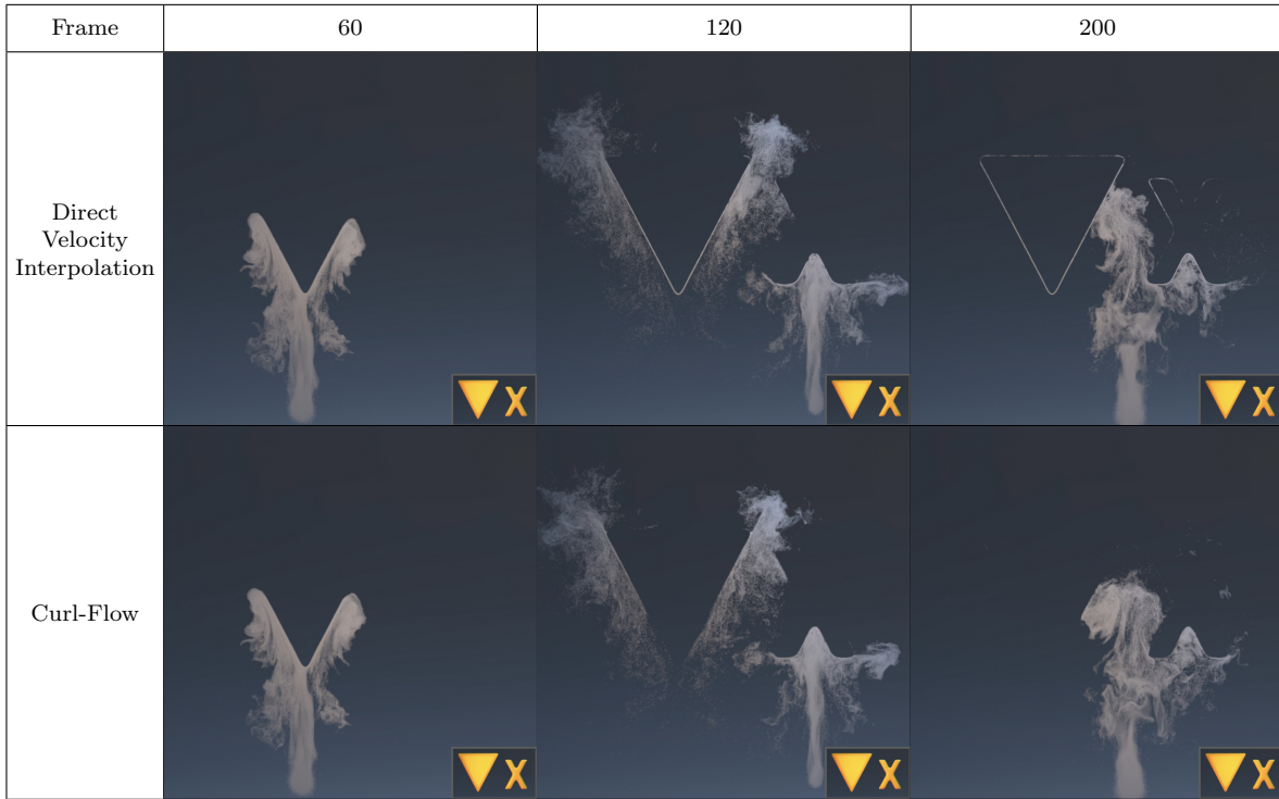
Figure 13.6: A Smoke Plume Simulation with A Solid Object Shaped like “ \nabla\times ”. Only a thin slice of smoke is visualized and the obstacles not rendered to better present the boundary behaviors. (The shape of the obstacles are shown at the bottom-right corner.) In the direct velocity interpolation case, a large number of particles erroneously collide with the solid leaving the dense smoke outline around the solid.
