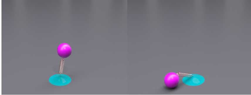
Figure 6.1: Toy Ball: A ball-and-spring toy composed of three point-connected parts. The behavior is different with proper point connection energies (left) in comparison with the one without any coupling energies (right). In the latter case, the sphere collapses to the ground.
