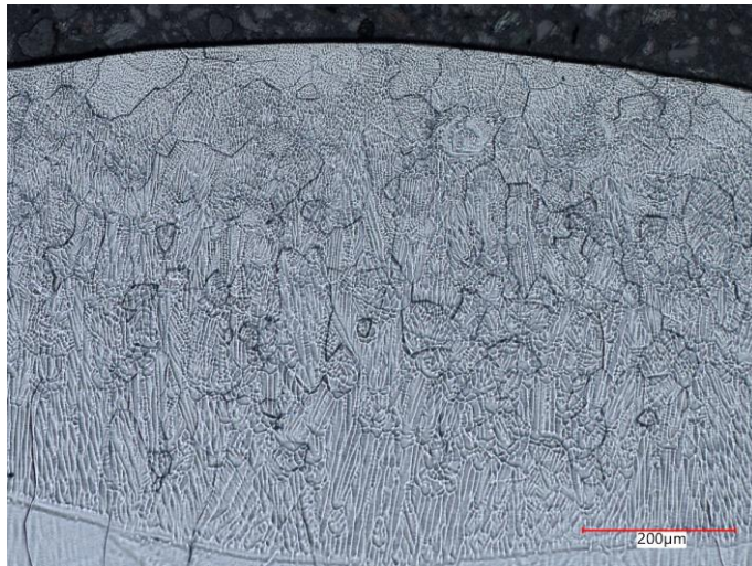
Figure 5-21. OM image showing the subgrain structure of track 16 (SP-2 sample) under the given processing parameter set ( P=600 W, F=6 g/min, v_i=10 mm/s and h_s=0.5 mm) and S-pattern scanning strategy.
