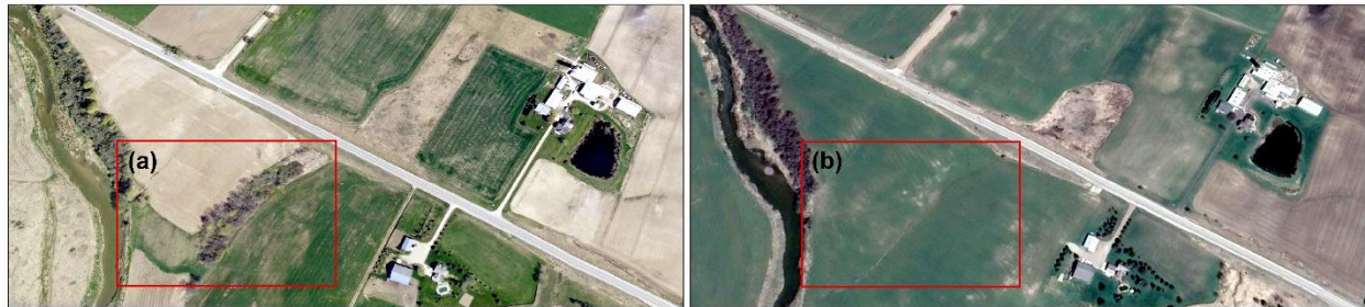
Fig. 6.5. Example of land cover change that resulted in an artificial drainage issue. Flow drains from the northern field into a culvert under a roadway that, (a) in 2006 drained into a tree and grass cover filter strip before entering the Nith River, and (b) in 2019 drains over another agricultural field directly into the Nith River, forming a large ephemeral gully annually. Source: SWOOP 2015 imagery (left) and Google 2019, Maxar Technologies (right).
