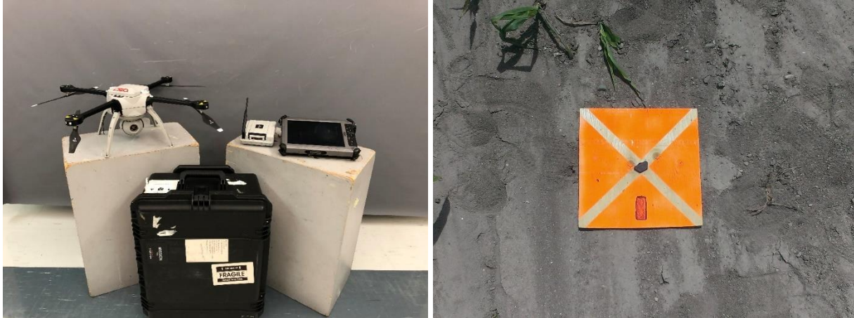
Fig. A1. Sphero R60 UAV system used for all data acquisitions (left) and a ground control point (GCP; right).
