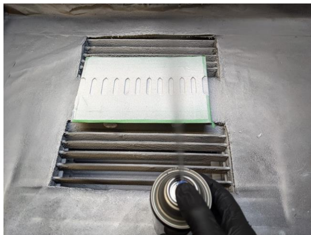
Figure 44. Speckling the tensile specimens with the black spray paint.
