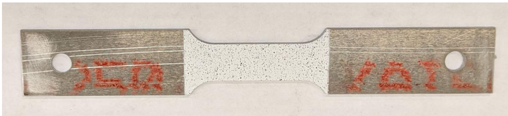
Figure 43. A tensile sample with black speckles on a white background, used to track the deformation of the gauge region using DIC.
