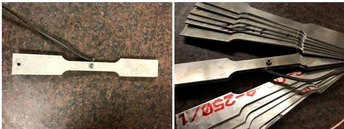
Figure 98. Instrumented tensile specimens used in the Sand Furnace.
