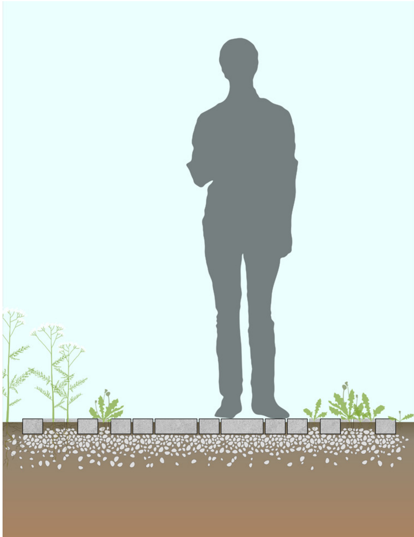
fig.47. Permeable Paving Section Detail
