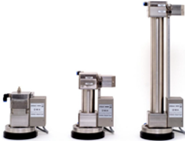
Figure 4.15: Small, medium, and large DMAs with different-sized columns [1]
