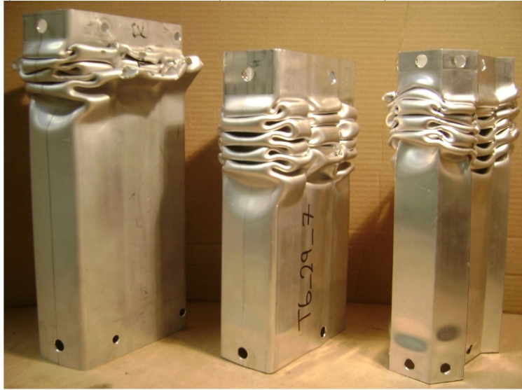
Figure 4.2: Experimentally crashed profiles [15]
