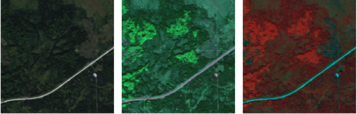
Figure 3.1: Left: RGB, Center: Red-Red-Edge-NIR, Right: Clipped NDVI
