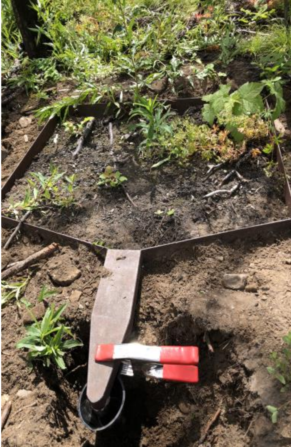
Figure 2.7: Rainfall simulation plot frame and sample collection setup with emerging vegetation at Site 5b.
