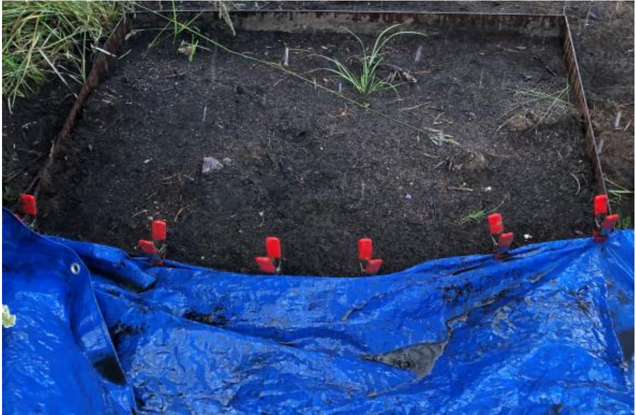
Figure 4.1: Rainfall simulation with unsaturated surface soil and ash layer at Site 4b.
