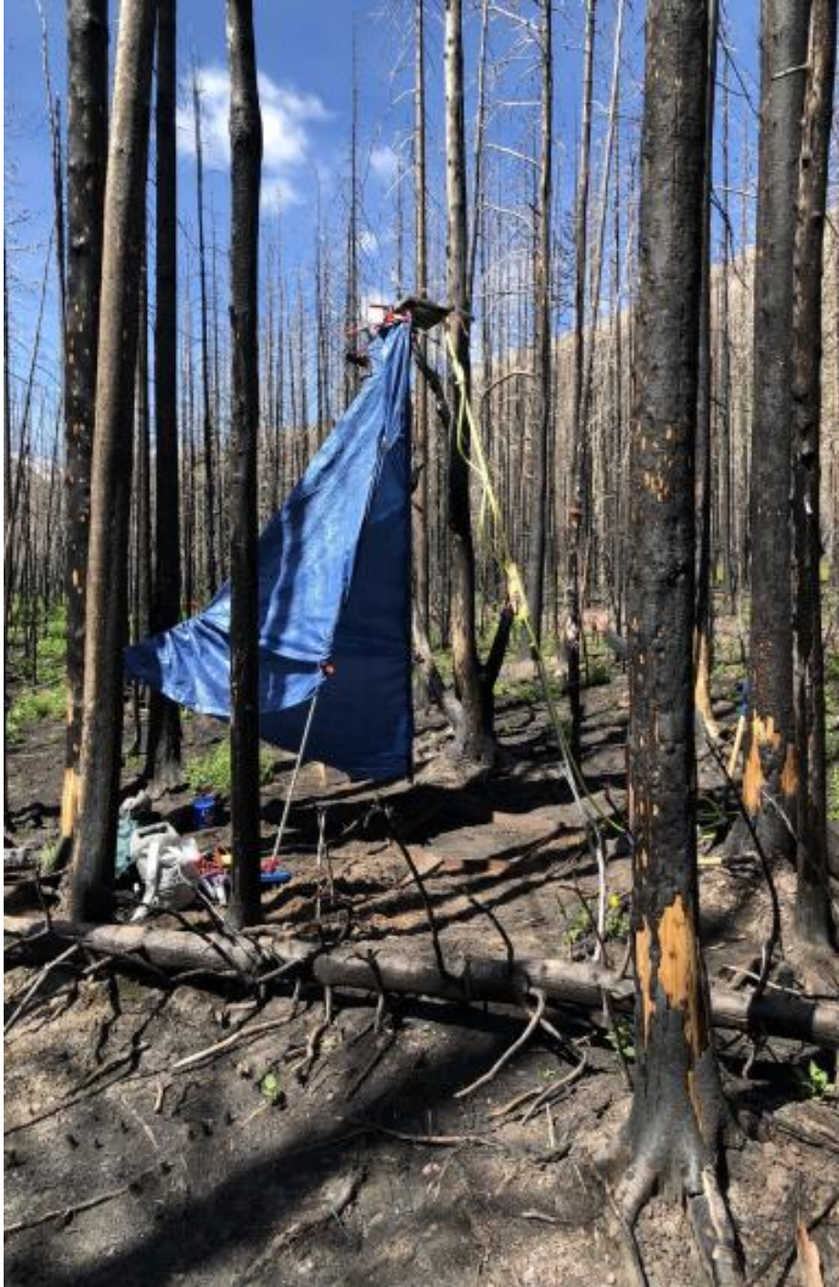
Figure 2.6: Rainfall simulator setup and design with windscreen at Site 10a.
