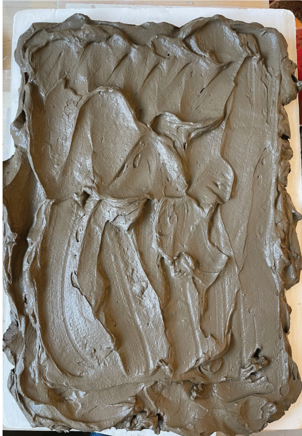
Figure 109. The clay must be dried on a plaster slab to a workable consistency.
