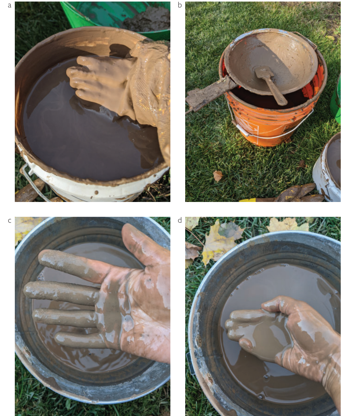
Figure 108. a-d. The processed wild clay is free of organics and very liquid.
