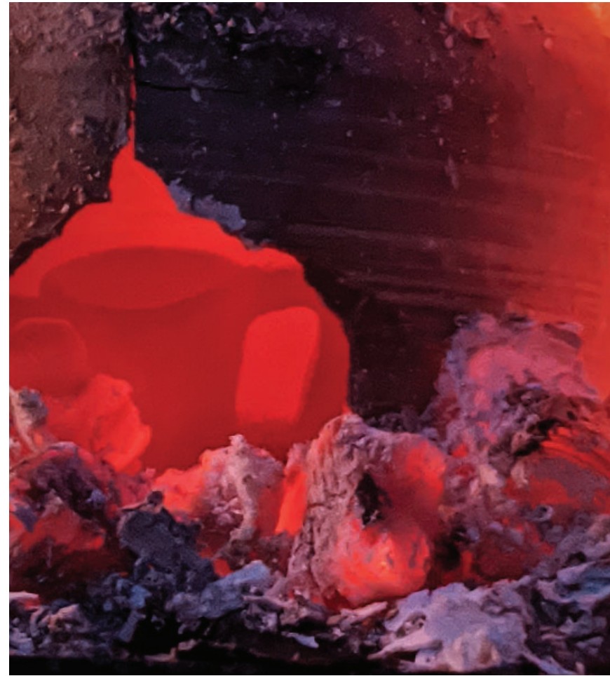
Figure 117. A wild clay pot glowing red in the heat of a pit fire.
