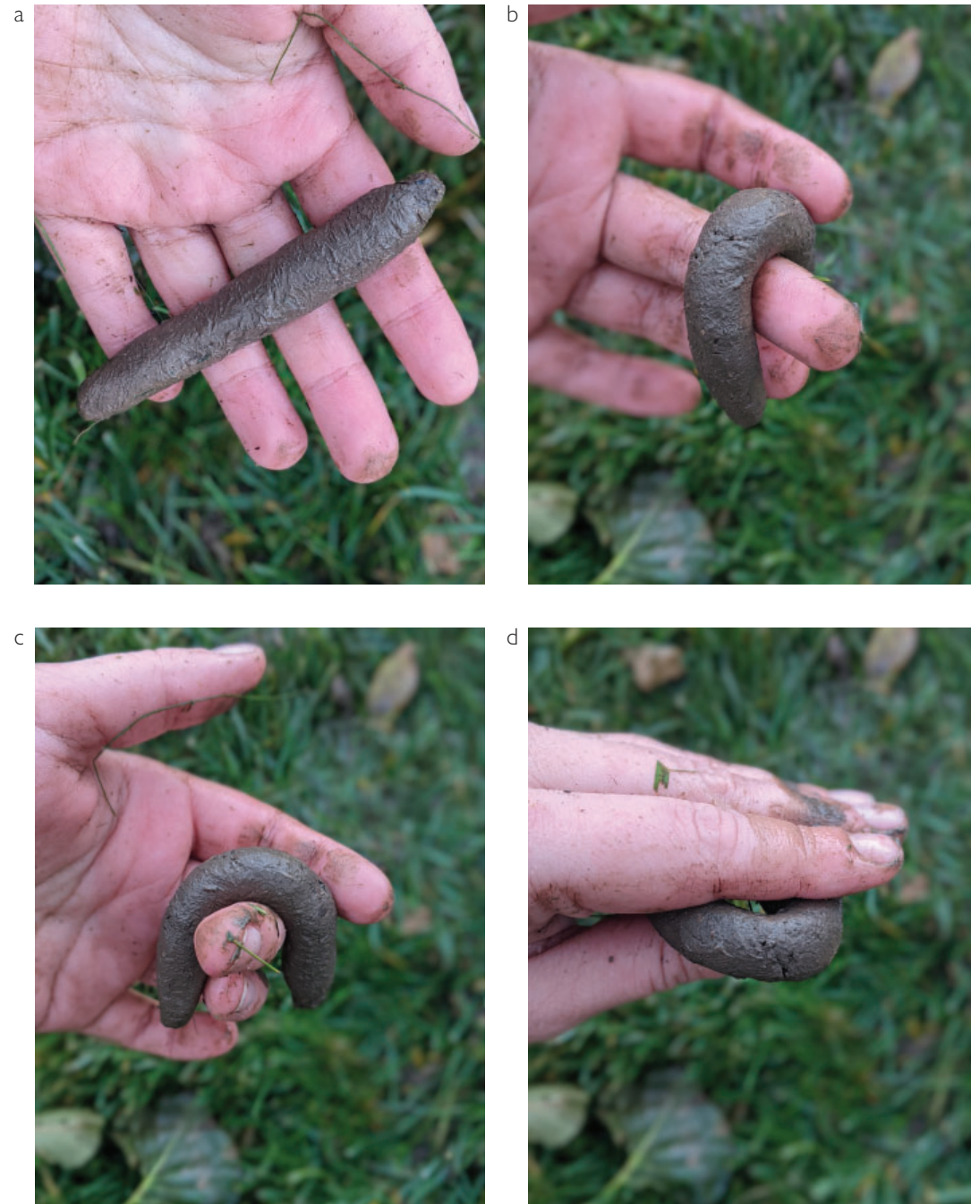
Figure 101. a-d. Images of a coil test on wild clay from Kitchener, Ontario. This clay does not crack when bent around a finger indicating it has the properties that are appropriate for throwing on the wheel.
