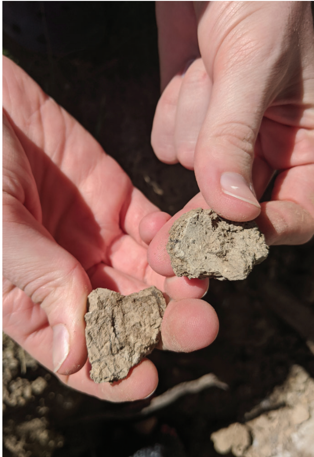
Figure 97. Snapping a chunk of dry soil to test if it will break along angular lines and reveal itself to be clay.
