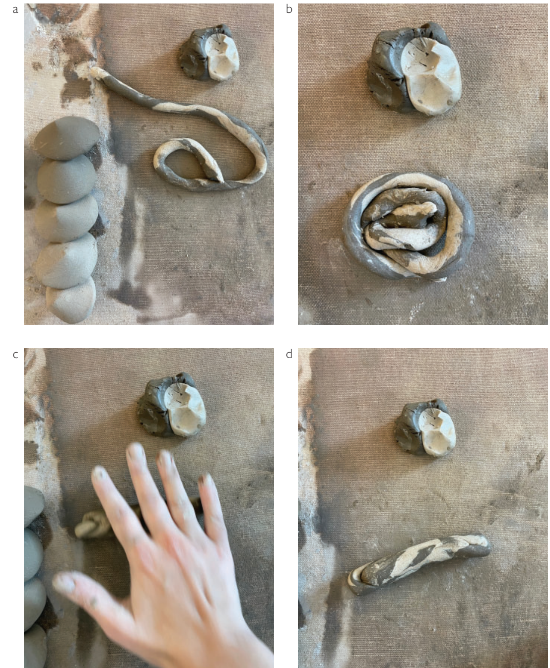
Figure 125. Coil wedging eases strain on wrists when wedging small amounts of clay. a. Roll ball of two clays into a long coil. b. Spiral coil up into a cinnamon bun shape. c. Roll out spiraled coil. d. Continue until ball of clay is homogeneous.
