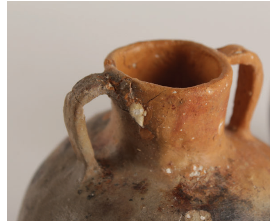
Figure 104. Lime Pop-Out tearing apart the neck of a vessel made of Komoka wild clay.
