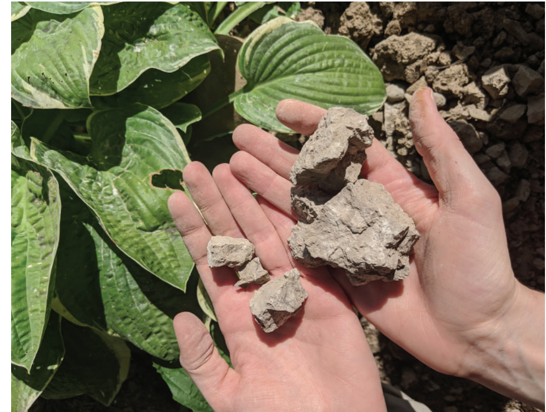
Figure 98. Dry clay with sharp edges mimics the shape of clay particles which are aligned in platelets.
