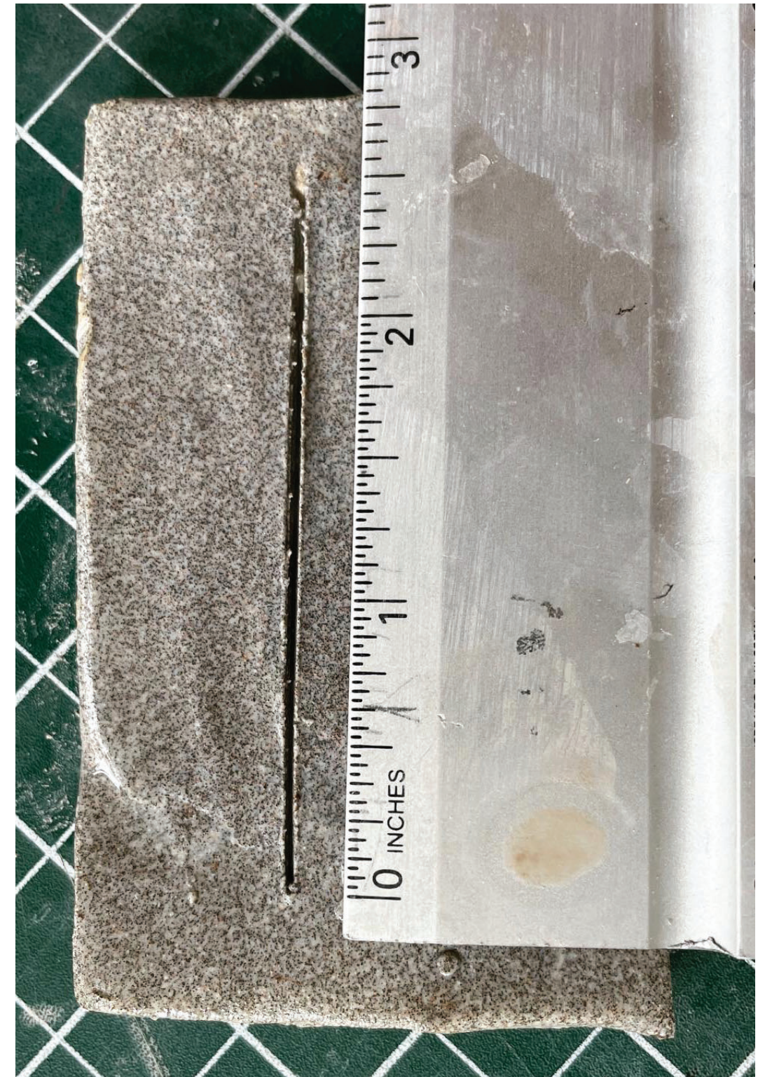
Figure 145. b. Marking a uniform dimension on raw clay test tiles allows for the calculation of the shrinkage rate post firing. This line measured 3" before firing and 2.5" post firing. By dividing the two measurements, I found this clay shrinks by 17%.
