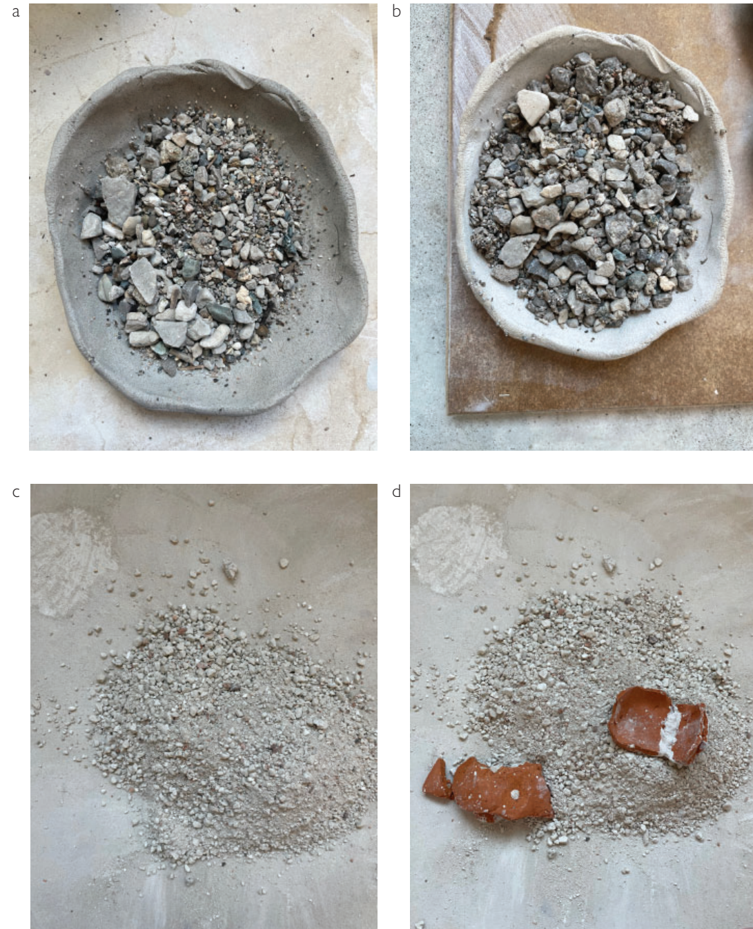
Figure 142. Calcine rocks to negate the effects of limestone by firing them to 1000°C. Make sure rocks are entirely dry before putting them in a kiln so they do not explode. a. Build a clay 'boat' to place rocks in for bisque firing. b. Rocks and boat post firing to 1000°C. c. Rocks can be easily crushed into powder after calcining. d. Mix limestone rock powder with water to form a quick setting mortar.
