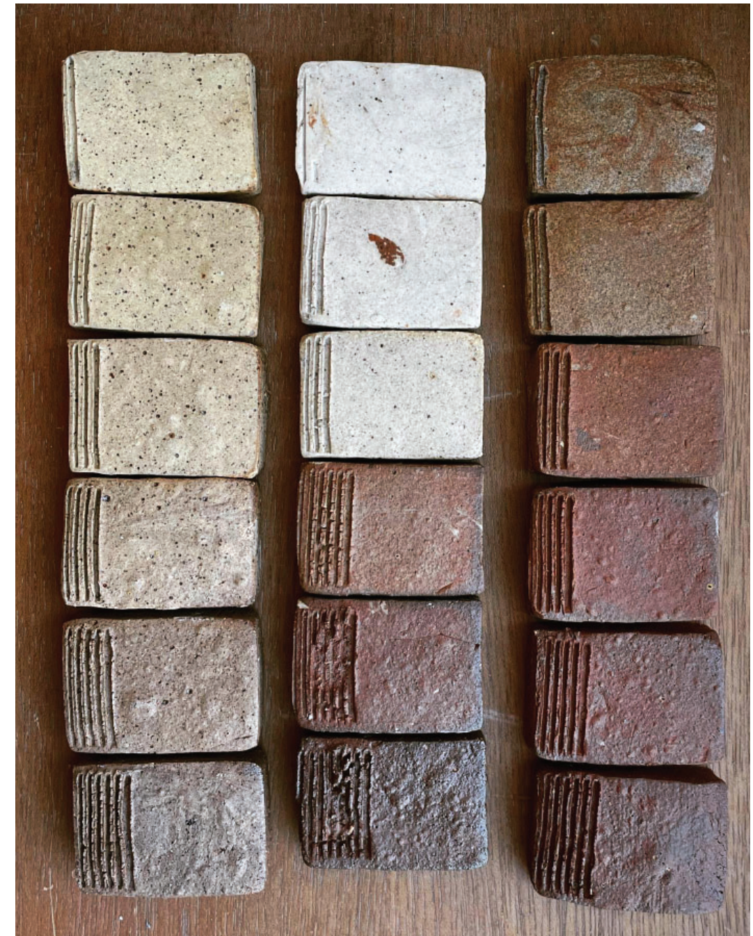
Figure 129. Test tiles lined up in accordance with their line-blend percentages.
