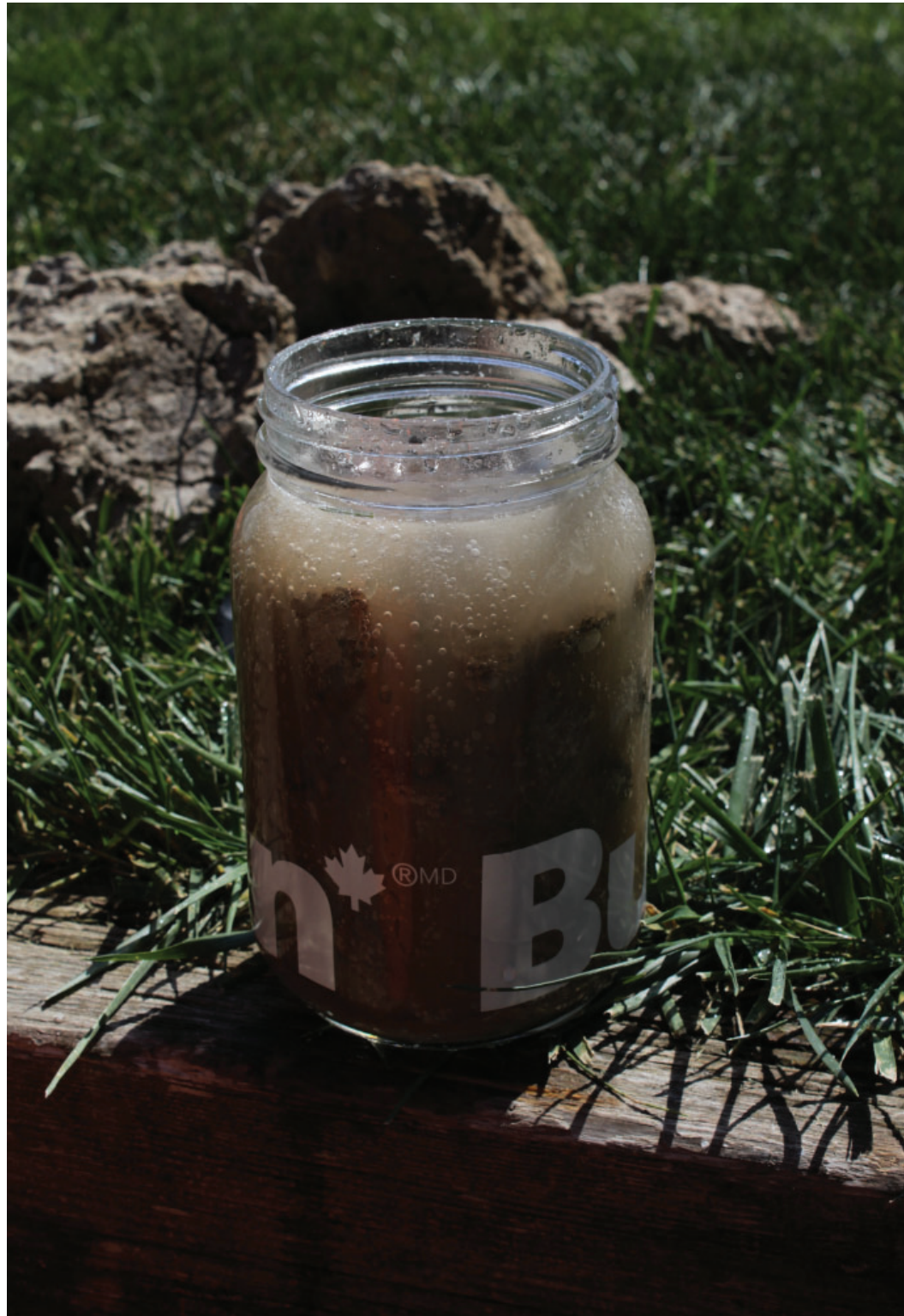
Figure 105. Testing for the presence of limestone in wild clay with vinegar and water.
