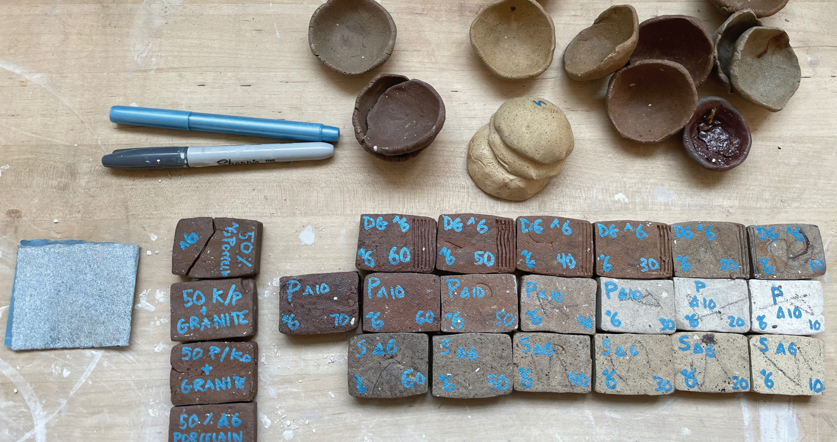
Figure 146. Documentation of the firing procedures and clay content values on the test tiles.
