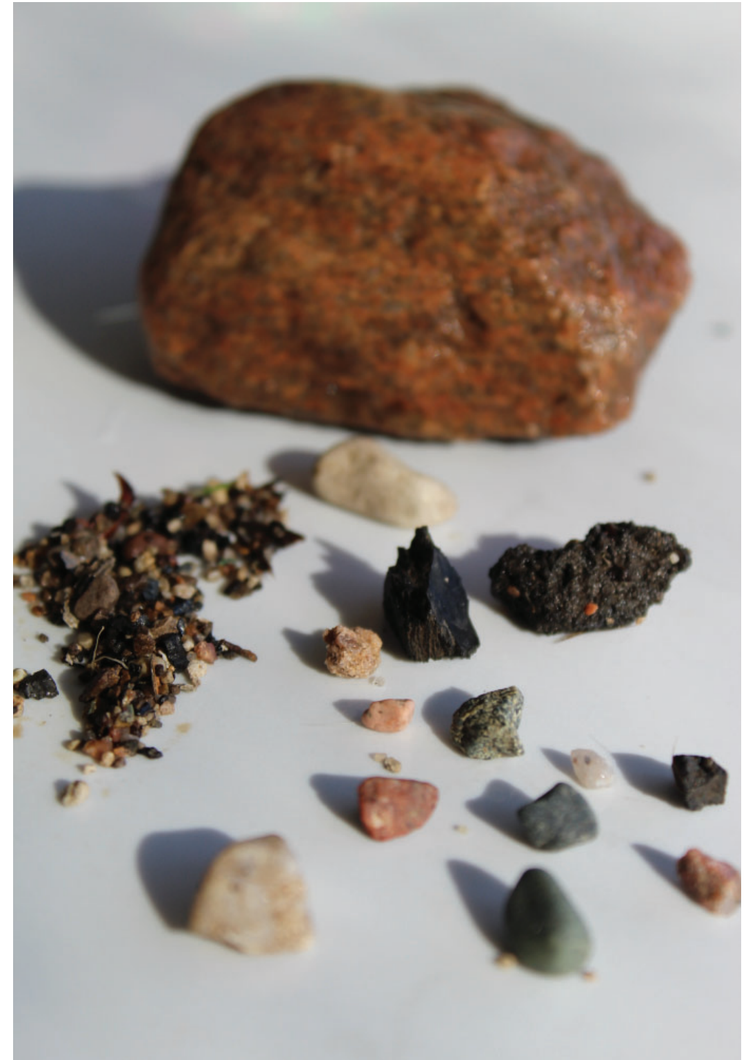
Figure 141. Various rocks pulled from the processing of the Kitchener clay.
