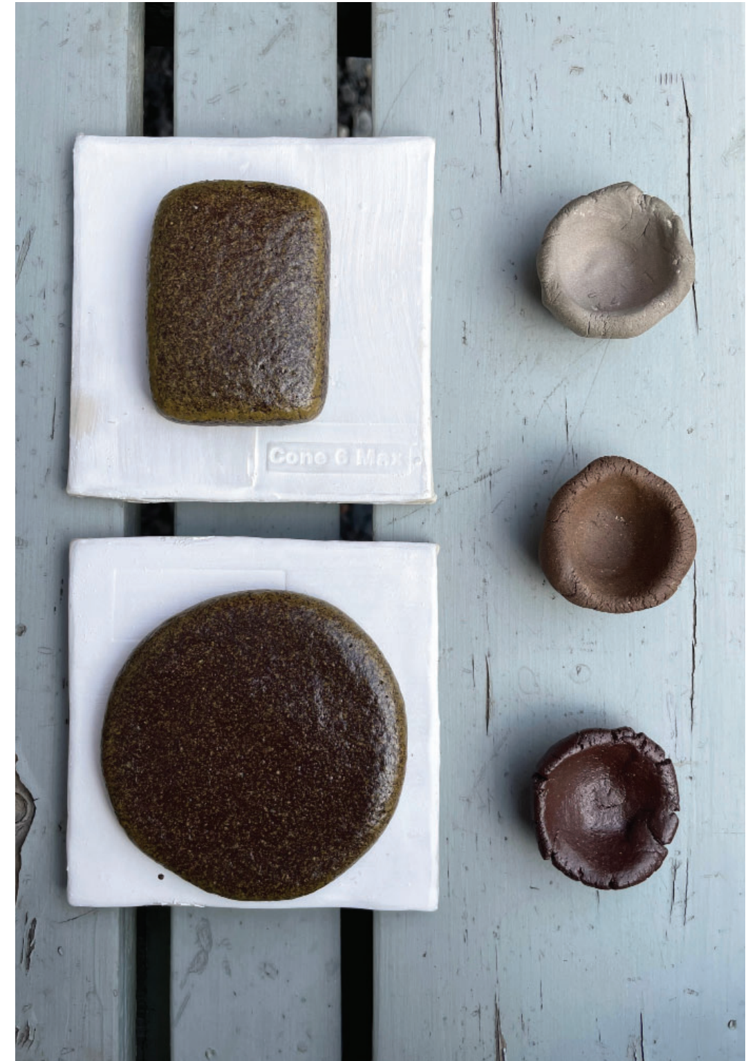
Figure 131. The Kitchener clay melted at cone 5, but the Trafalgar clay held its shape.
