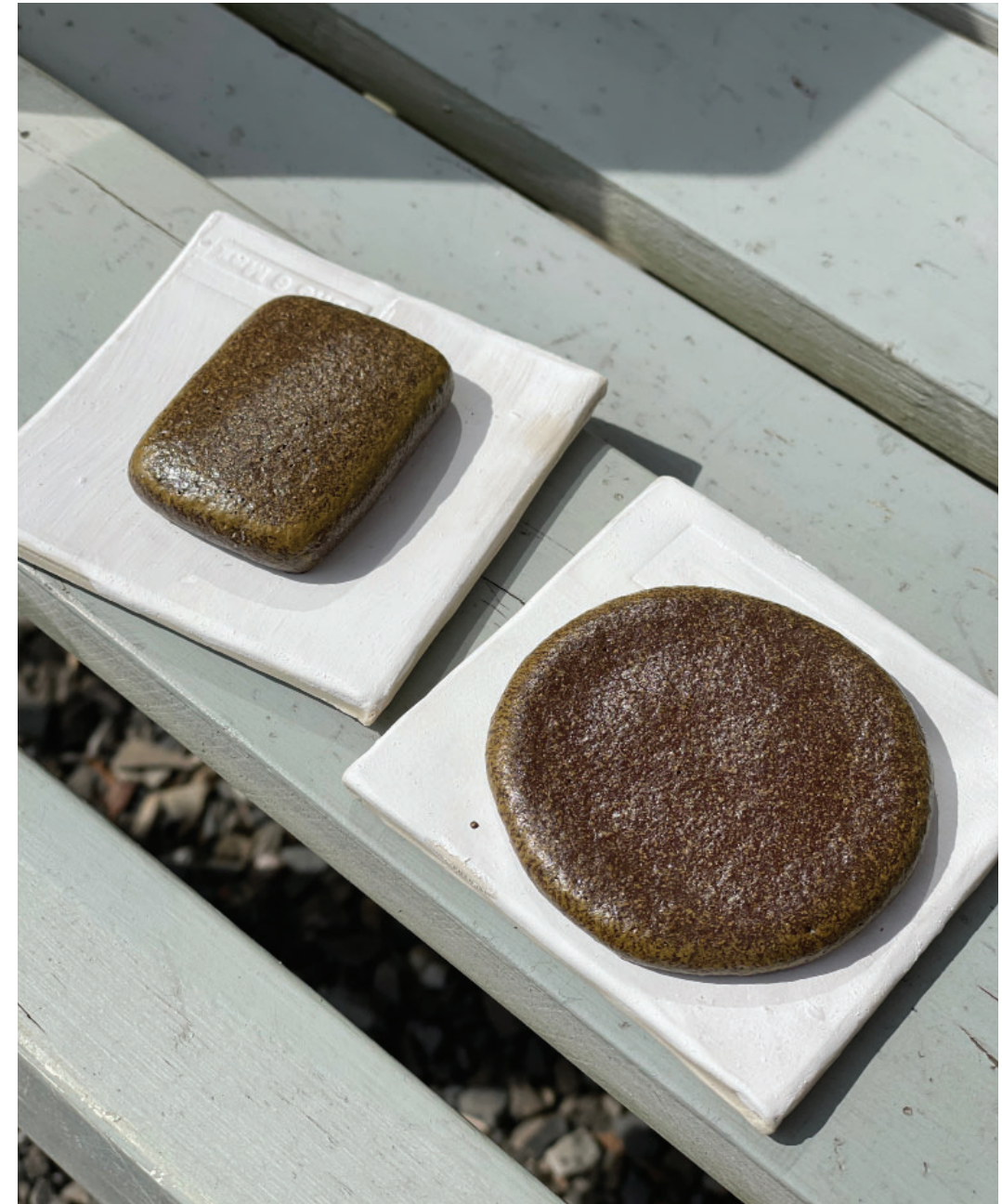
Figure 138. Melted test tile and pinch pot made from Kitchener clay when fired to cone 5.
