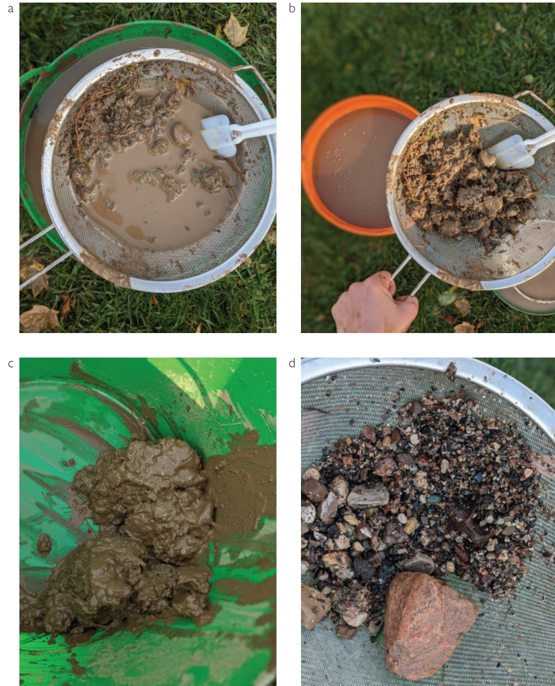
Figure 107. Processing wild clay. a. Strain the watered down wild clay through a mesh screen b. The organic material left after screening c. Deposit organics in a bucket d. Wash organics and rocks and set aside.
