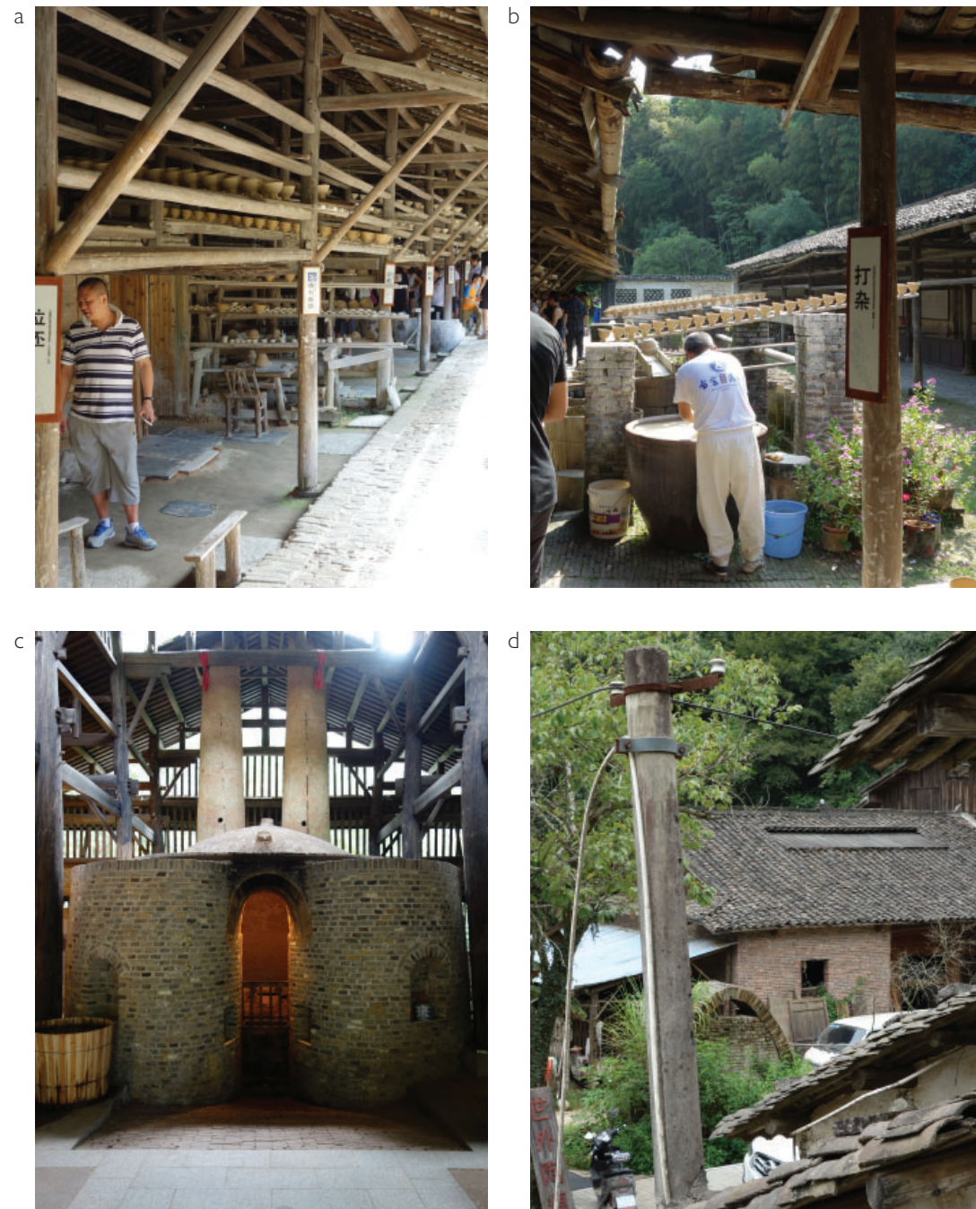
Figure 64. Places of ceramic production in Jingdezhen. a. Ware drying in the rafters b. Bowls drying in the sun c. A kiln with two smoke stacks d. Ceramic roof tiles in the foreground and a catenary arch kiln in the background
