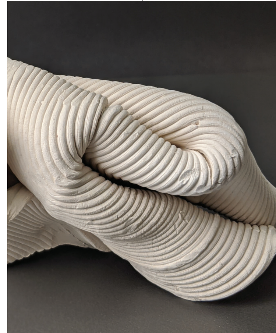
Figure 21. Collapsed 3D printed clay vessel, folded upon itself. Printed in the fall of 2019 as part of the Material Syntax elective at the School of Architecture in Cambridge, Ontario.
