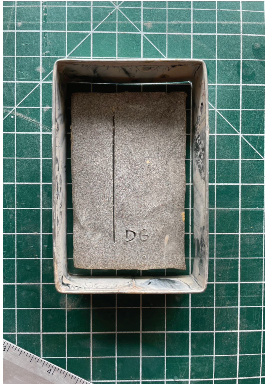
Figure 145. a. Clay test tile sitting within the cookie cutter used to shape the tile showing the shrinkage. Information gathered from Mitch Iberg and Zoe Powell, "Clay Processing Workshop Guide," 16.
