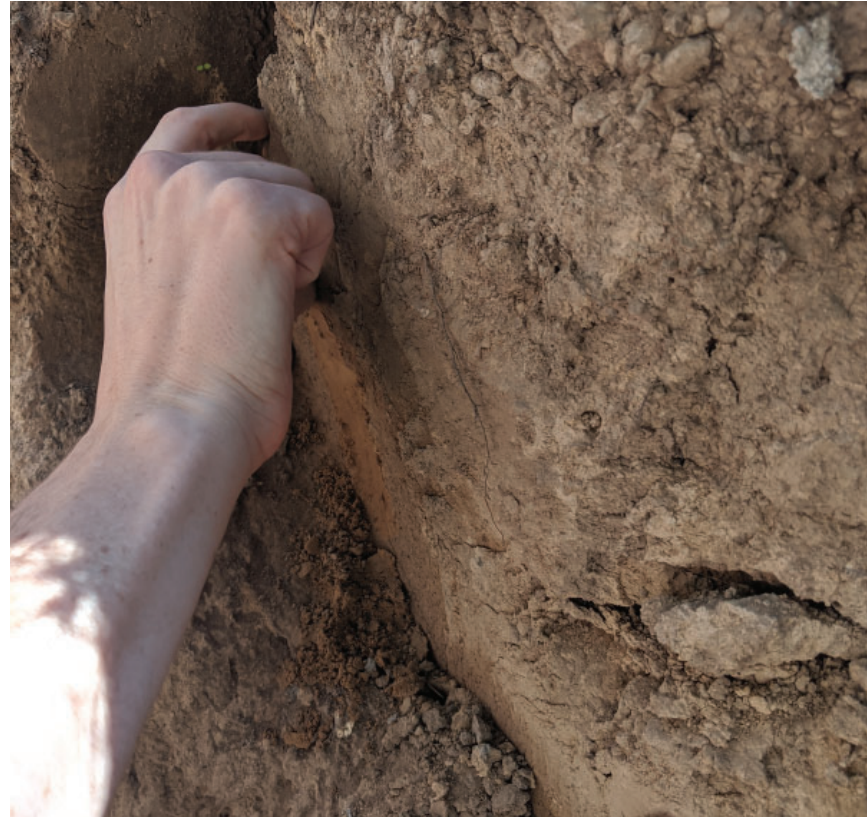
Figure 14. Clay found during an foundation excavation in Komoka, Ontario.
