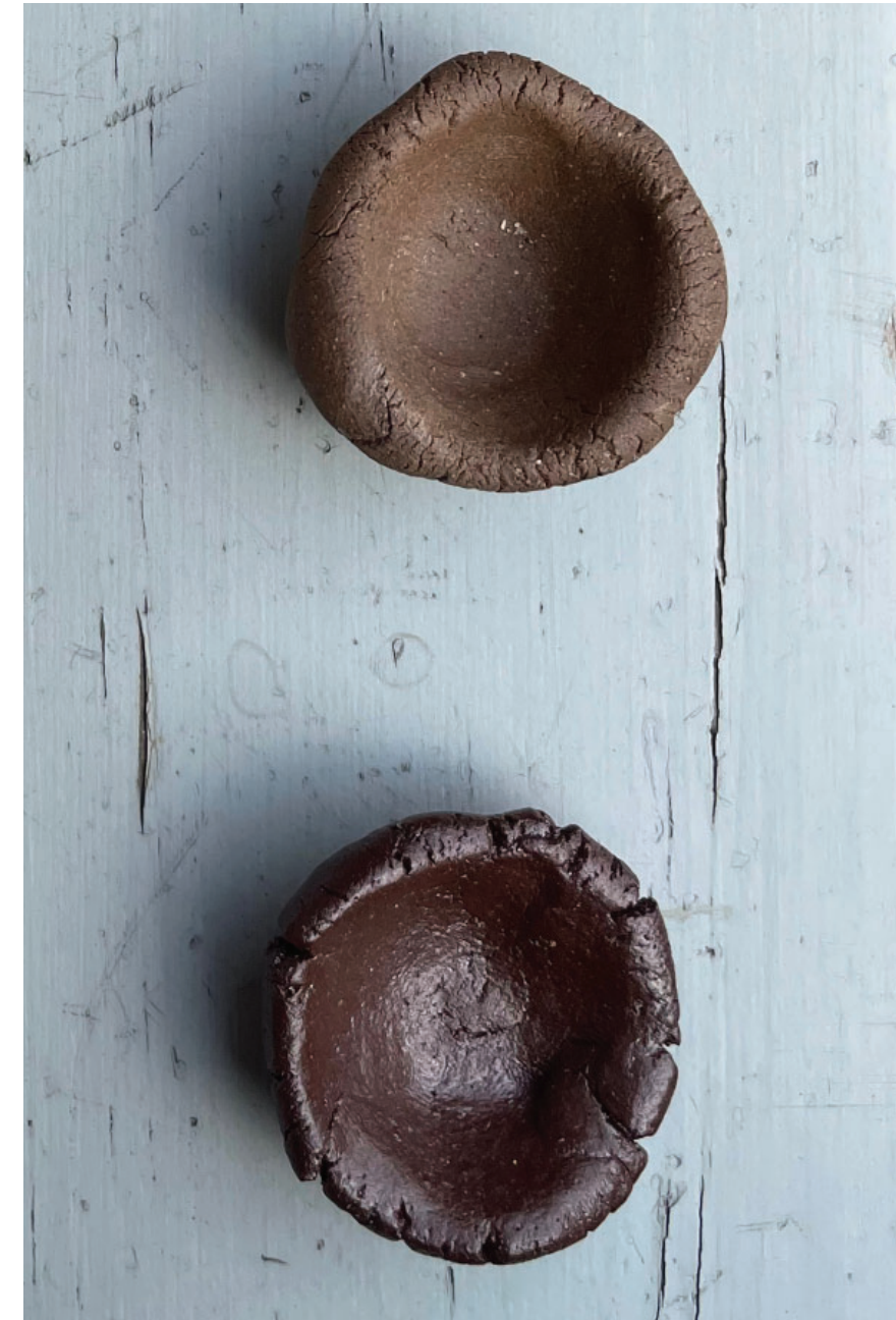
Figure 136. Top: 50% Trafalgar clay, 50% porcelain fired to cone 5. Bottom: 100% Trafalgar clay fired to cone 5.
