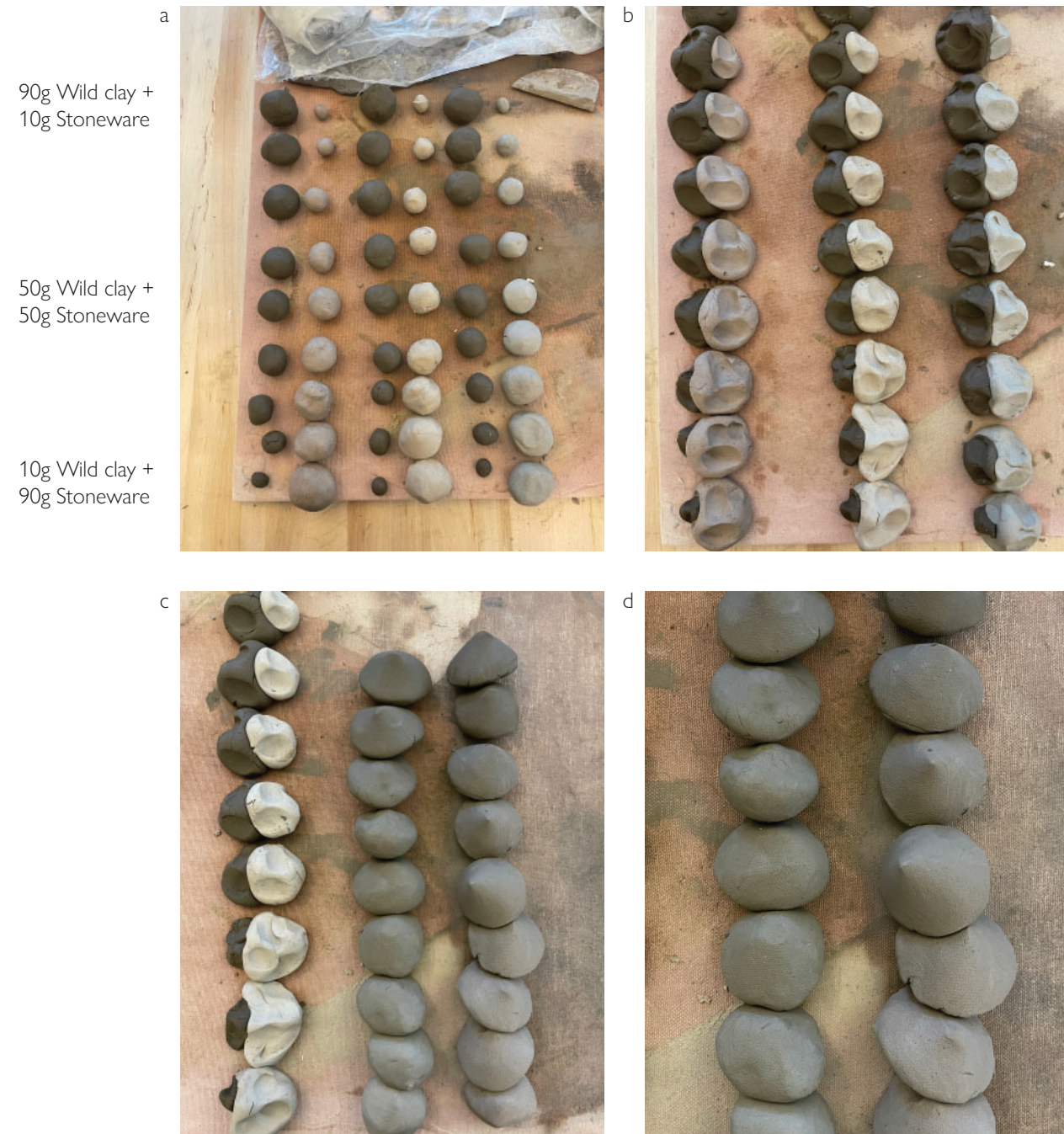
Figure 124. Making line-blend test tiles. a. Weigh out 100g balls in descending percentages to combine two different clay bodies. b. Combine the balls together. c. Wedge the two clay bodies until homogenous. d. Wedged balls of clay lined up in order of percentage change.
