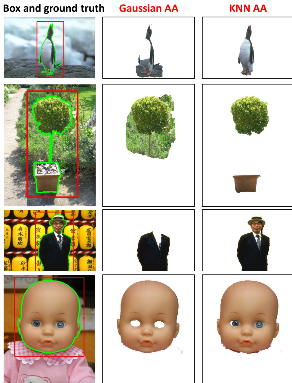
Figure 3.8: Representative interactive segmentation results. Regularized average association (AA) with fixed bandwidth kernel (3.1) or adaptive KNN kernels (Example 3.3) is optimized as in [281]. Red boxes define initial clustering, green contours define ground-truth clustering. Table 3.1 provides the error statistics. Breiman’s bias manifests itself by isolating the most frequent color from the rest.
