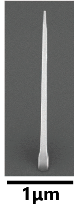
Figure 2.2: SEM image of a tapered InP nanowire waveguide. The quantum dot is embedded 200 nm from the base. Image from [60] licensed under CC BY 4.0.
