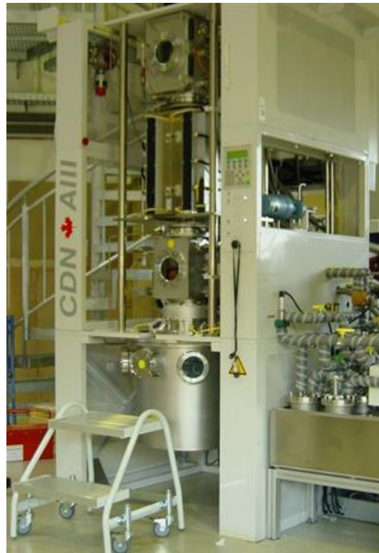
Figure 4-2. McMaster galvanizing simulator used to anneal the samples in present work.
