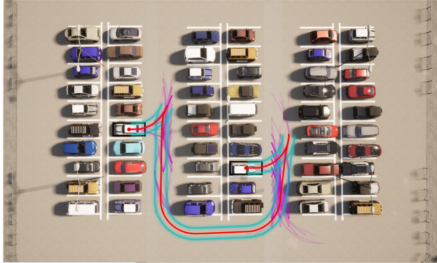
Figure 5.9: Motion planning using t -spanning G^3 motion primitives. Magenta: primitives used, Red: final motion, Cyan: car footprint.
