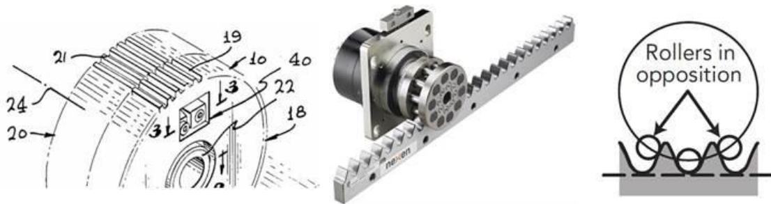
Figure 2.22 Split pinion [206] (left); Existing variations of rack and pinion [209] (right).
