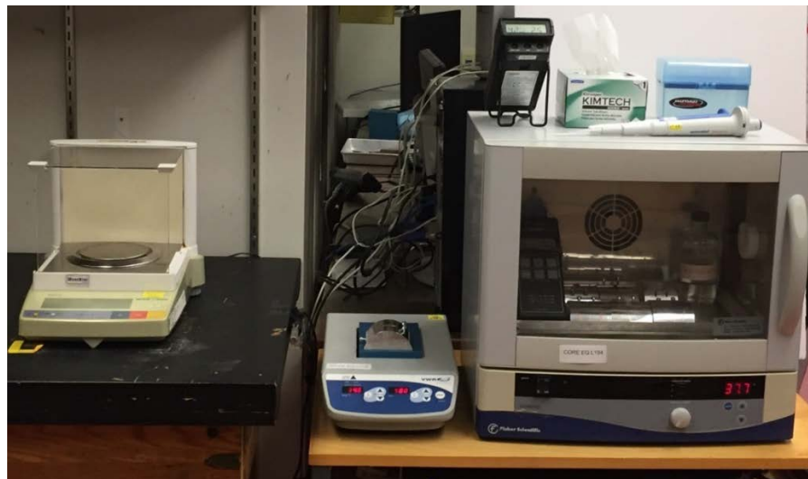
Figure 3-3: Experimental set-up for water loss measurements with an analytical balance, heating plate, model eye, and oven (left to right).
