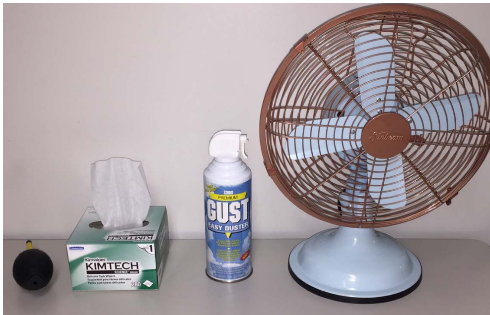
Figure 6-12: Different methods of ventilating the evaporimeter.
