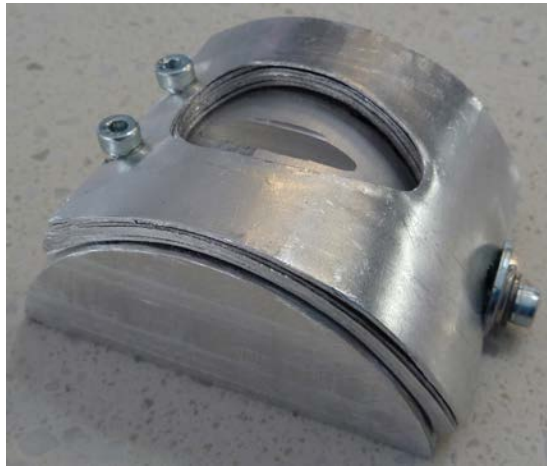
Figure 3-15: Aluminum inserts placed on the model eye to increase the air volume inside the evaporimeter.
