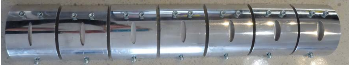
Figure 3-14: Elliptical model eyes with surface areas of 1 cm 2 to 2.5 cm 2 (left to right).
