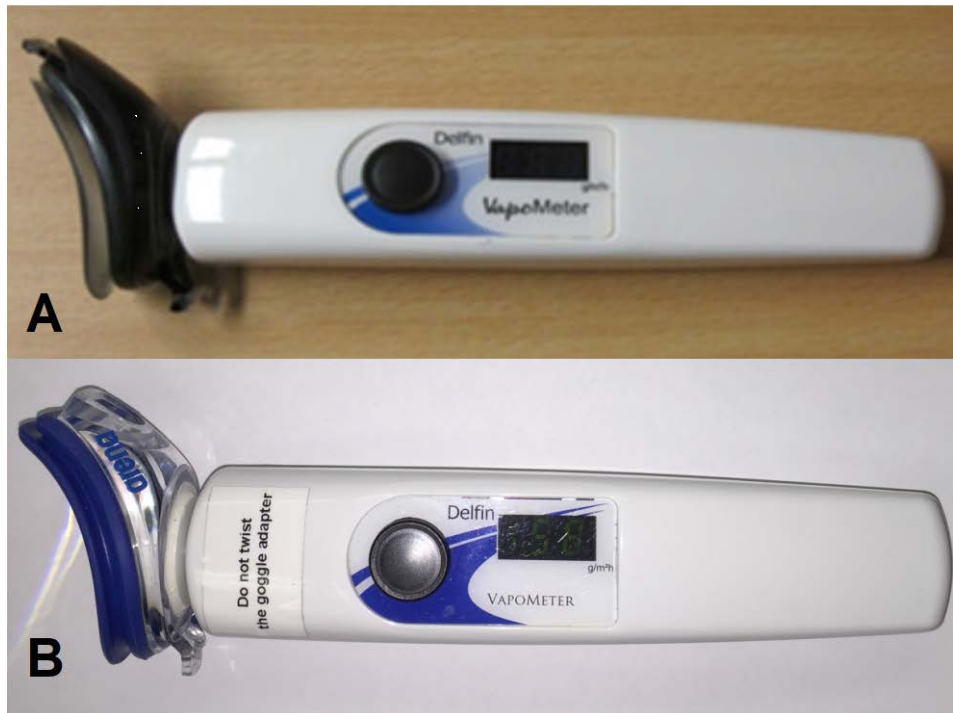
Figure 3-1: Original goggle and instrument used to validate the Eye-VapoMeter (A) compared to the commercially available instrument (B). Image A from Rohit A, et al. Validating a new device for measuring tear evaporation rates. Ophthalmic Physiol Opt. 2014;34:53-62.
