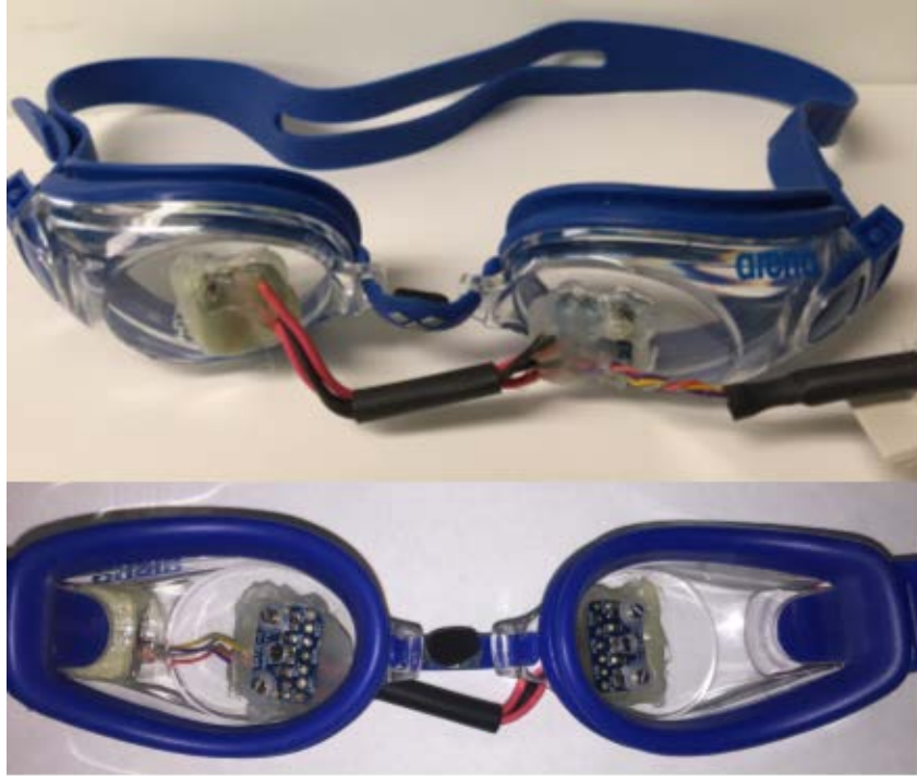
Figure 4-1: View of the evaporimeter with a sensor attached to the front surface of each goggle, as seen from the front (top) and back (bottom).
