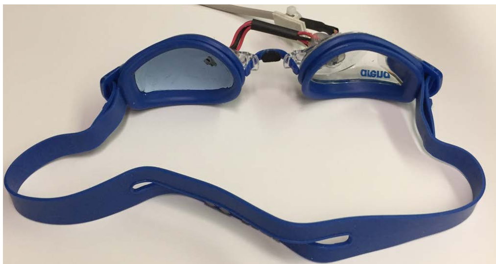
Figure 5-1: Modelling clay inserted into the right goggle to decrease the volume inside the evaporimeter.
