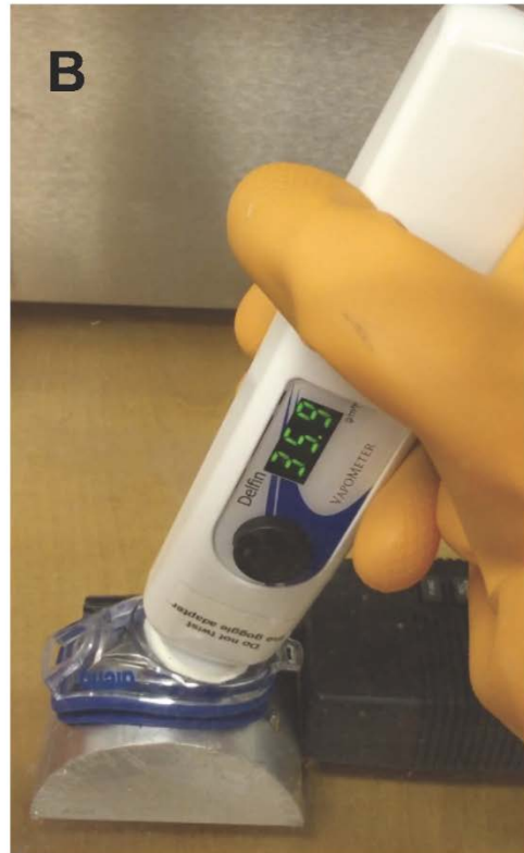
Figure 2-1: Placement of a soft contact lens with the back surface against the model eye (A), with a red outline highlighting the location of the soft contact lens. The black line outline shown in (A) helped align the Eye-VapoMeter over the model eye (B) to ensure the instrument was held in the same position during each measurement.
