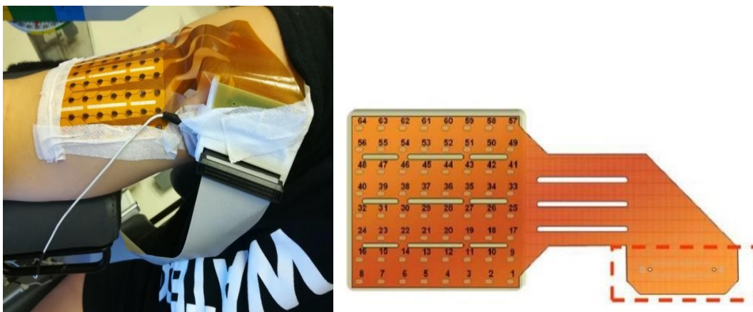
Figure 3: High Density sEMG (HD-sEMG) electrode grid placement on subject and numerical reference of the electrodes.
