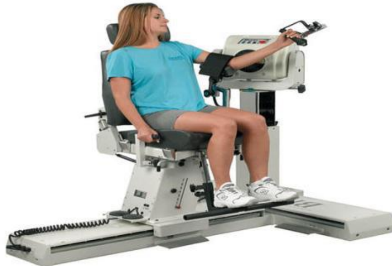
Figure 4: Dynamometer system during elbow flexion. Arm constraint was removed throughout the protocol to allow for placement of HD-sEMG electrode grid. Taken from [82].
