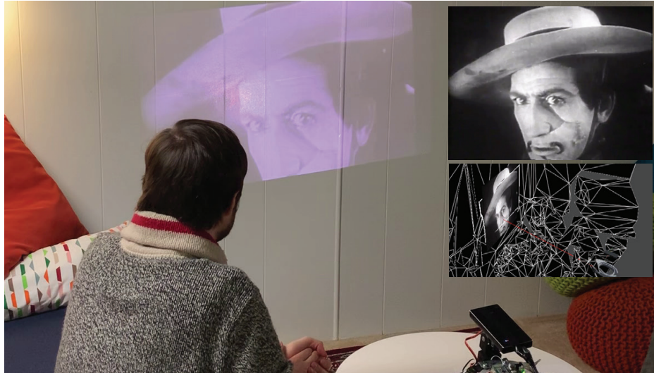
Figure 6.2: AR persistence example application. The projector acts as an ad hoc display when the user takes off the HMD, enabling them to continue watching a video started in AR.
