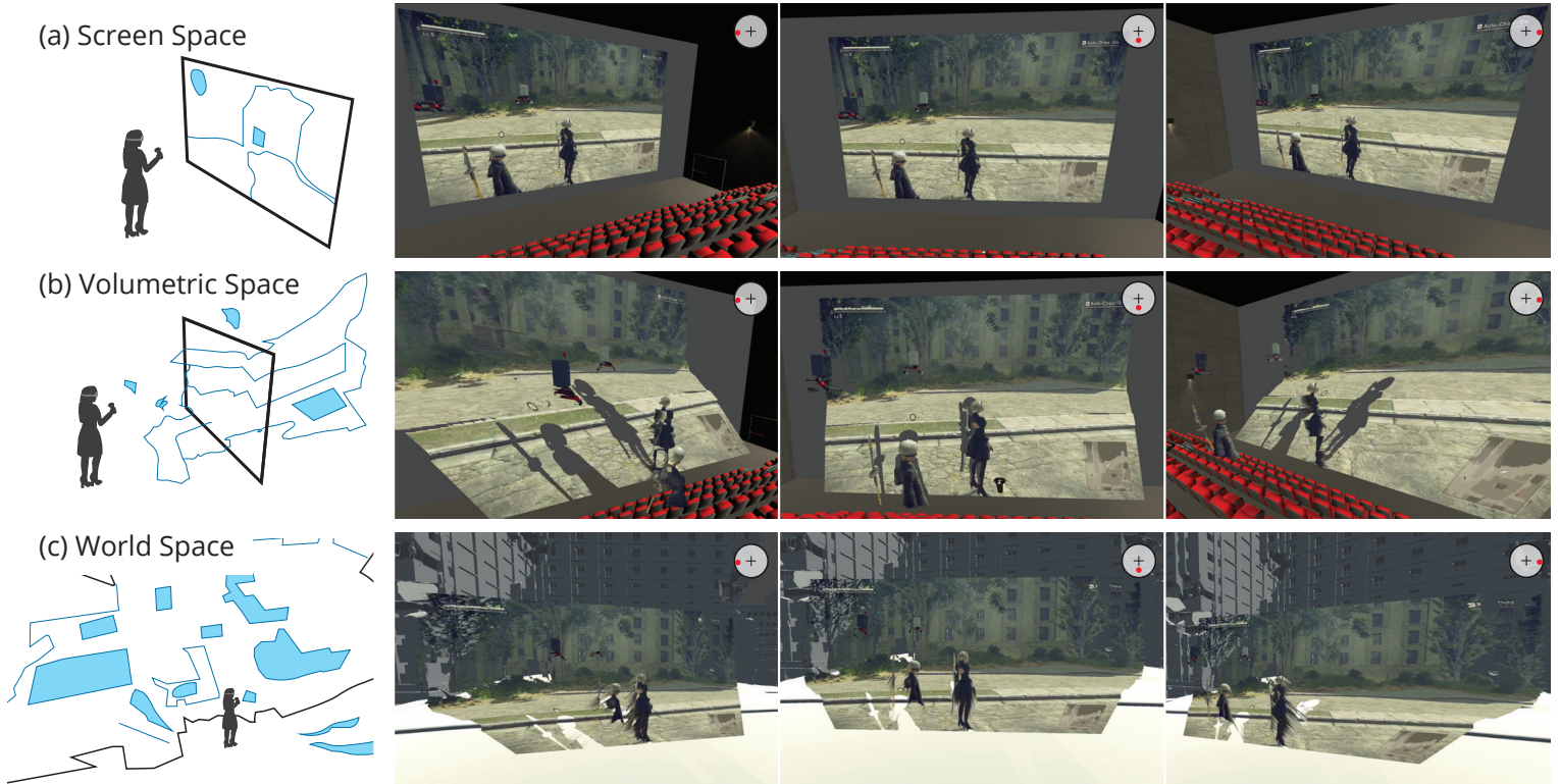
Figure 7.2: Spectator experience levels: (a) screen space view uses the 2D video frames from the stream; (b) volumetric view uses the depth data to provide a 3D effect with limited locomotion and interaction; (c) the world space view uses both the depth data and low-fidelity models from the game to create an environment that maximizes the spectator's locomotion and interaction capabilities.
