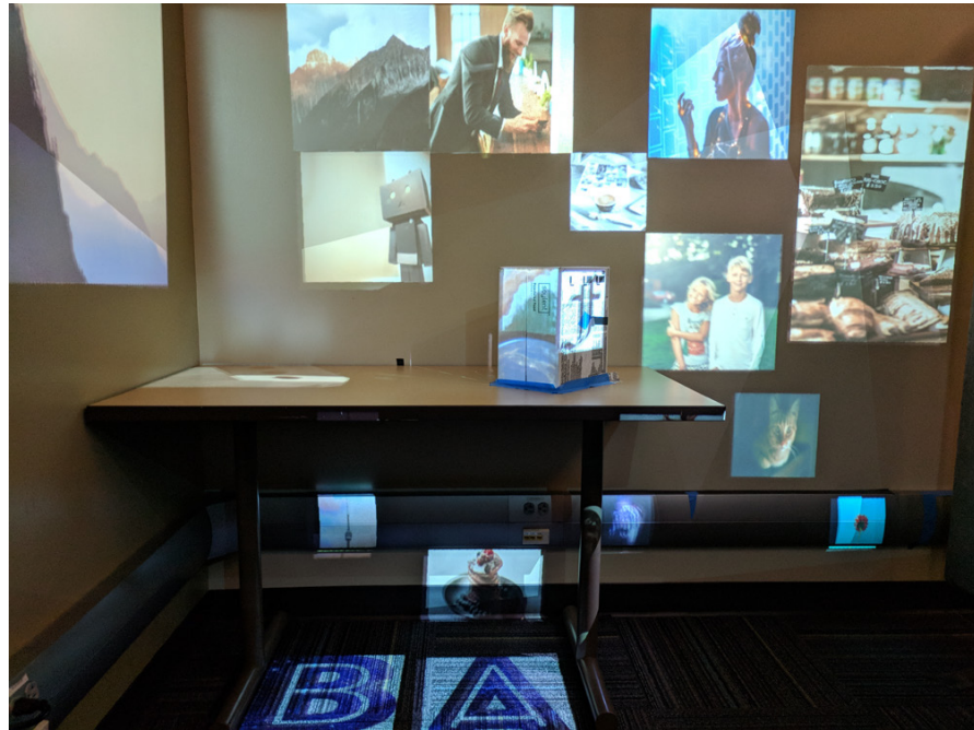
Figure 4.4: An example of spatially distributed content viewed in a SAR setup. Note how content can be displayed on any surface including walls, floor, furniture, and objects.
