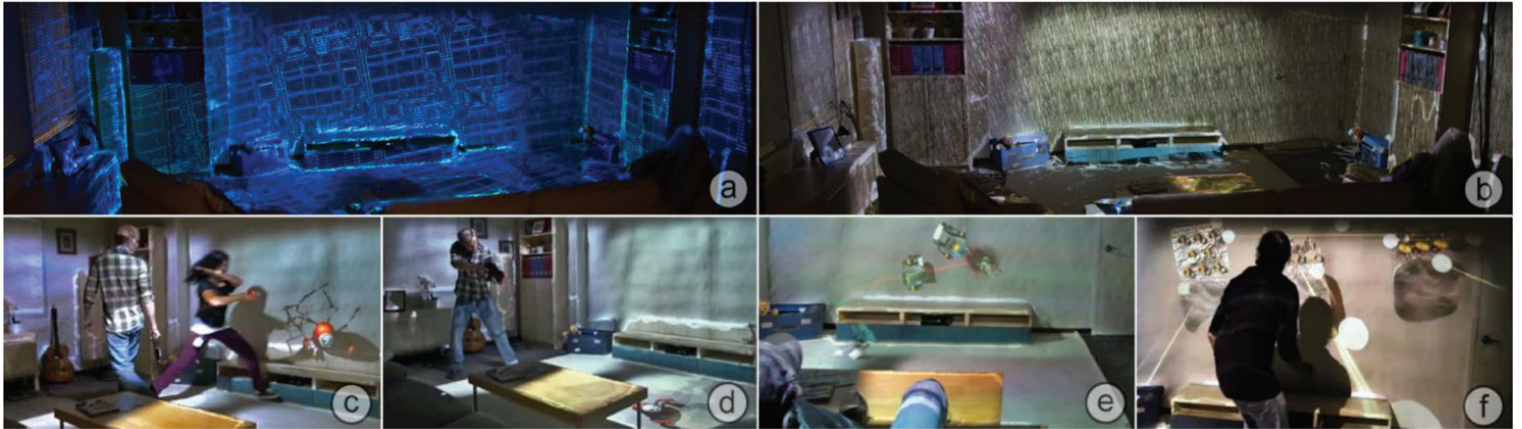
Figure 2.3: RoomAlive uses projection-mapping to create an immersive spatial augmented reality environment. Images (a) to (f) showcase how the same room can be augmented using different virtual scenes (from Jones et al. [114]).
