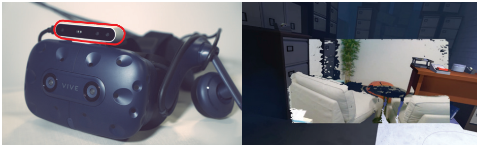
Figure 5.6: HTC Vive with Intel RealSense highlighted in red (left). The composited depth image with a virtual scene (right).
