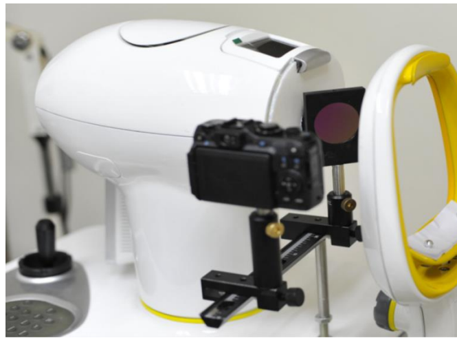
Figure 2-10: Dual camera system using a semi-reflecting germanium beam-splitter to permit simultaneous visible and IR imaging of the eye surface, Su et al. 69 (Reproduced from: Su T, Chang S, Yang C, Chiang HK. Direct observation and validation of fluorescein tear film break-up patterns by using a dual thermal-fluorescent imaging system. Biomedical optics express . 2014;5(8):2614-2619)
