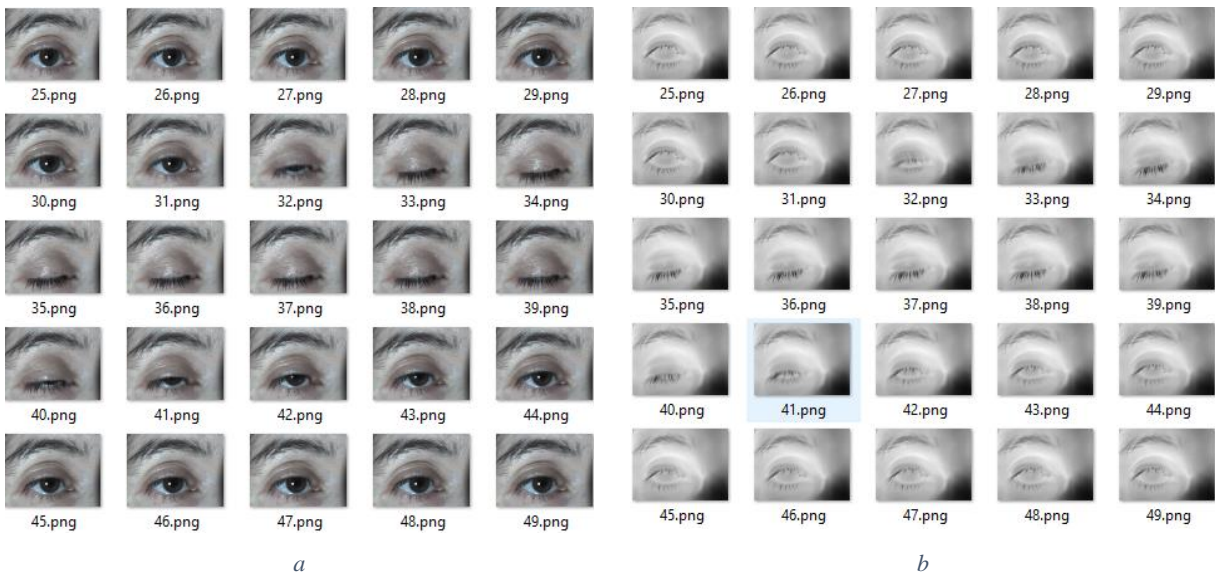
Figure 3-10: Visible (a) and thermal (b) extracted video frames used for side-by-side comparison, numbered from an initial reference frame.
