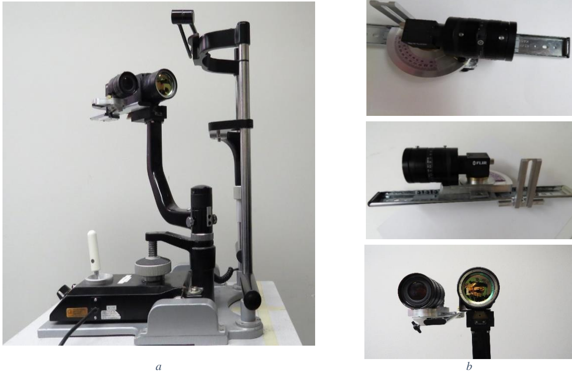
Figure 3-4: a) Mounting arrangement for the two cameras showing the movable arm mounted on the slit-lamp biomicroscope, the camera mounting and the subject headrest, b) different views of the visible camera mount (top, middle) that was attached to the thermal camera (bottom).
