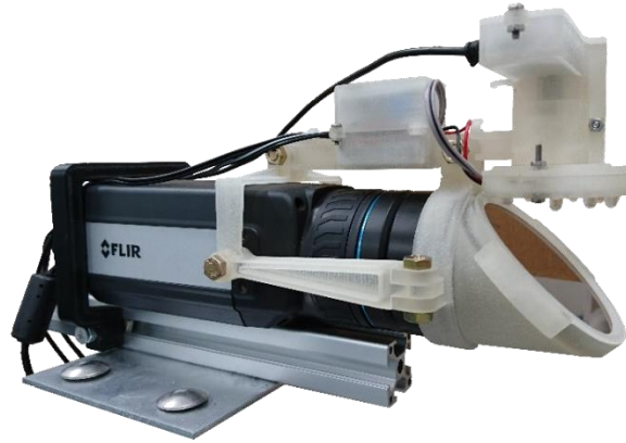
Figure 2-12: New camera installation using semi-reflecting Germanium beam-splitter introduced by Kricancic et al. 71 (Reproduced from: Kricancic H, McNeill H, Titze M, Alonso-Caneiro D, Collins MJ. Instrument for simultaneous assessment of fluorescein and thermal dynamics of the tear film. 2017)
