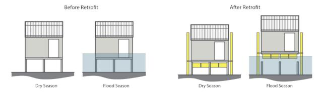
Figure 1.31. A building retrofitted with buoyant foundation. Source: Bullough, Khokhar & English, 2019.
