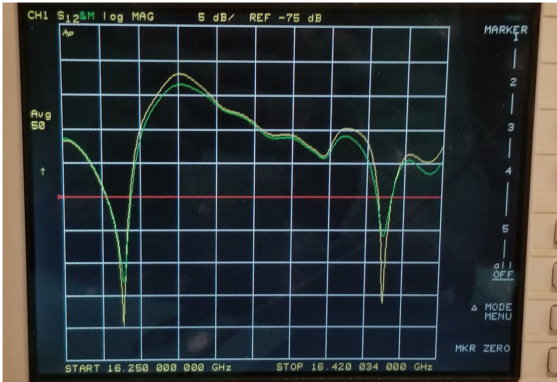
Figure 4.5: Transmission response of superconducting (Yellow) and non-superconducting (Green) niobium resonator. Two peaks are observed: one at f = 16.27 GHz and one at f = 16.39 GHz. Both appear to be related to the Nb on the PCB as they both increase in transmission when the resonator turns superconducting. However, the resonance dip at f = 16.39 GHz is expected to result from the resonator itself as the Q-factor also changes.
