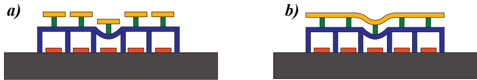
Figure 1.12: a) Segmented DM, b) Continuous DM [42]. Copyrights© 2011. Springer Nature.
