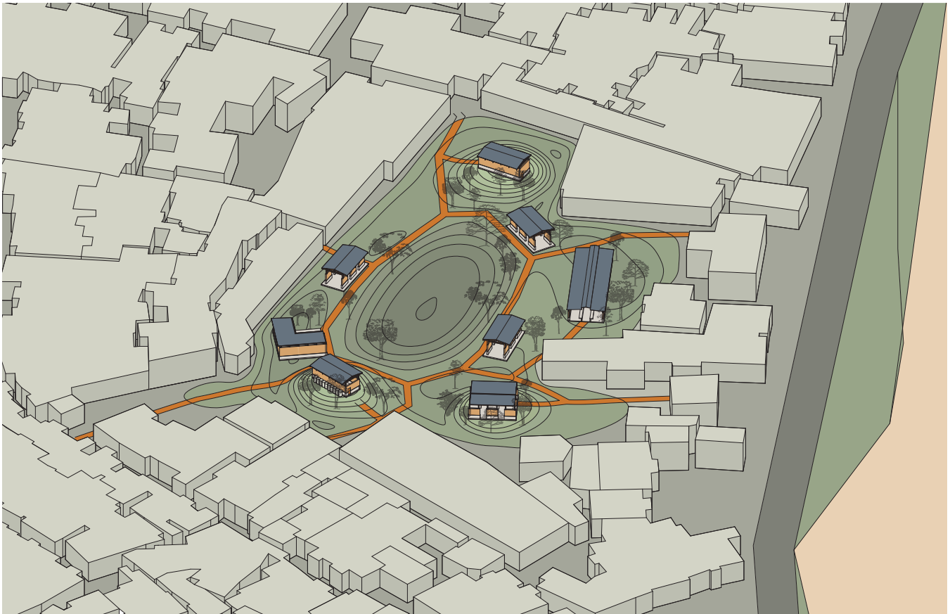
Fig. 4.30 Isometric of Site 2 flood-adaptive public space. This site has a total area of 8,022 m 2 and an effective capacity of 8,565 m 3 .
