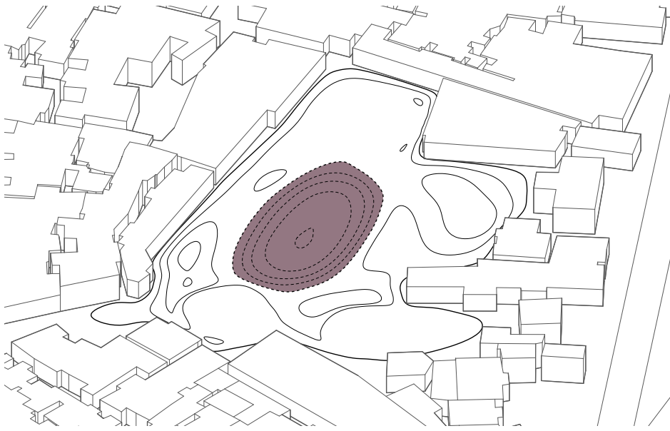
Fig. 4.32 The central area will be excavated to be the main flood storage. Total excavated soil has a volume of 2,190 m 3 .
