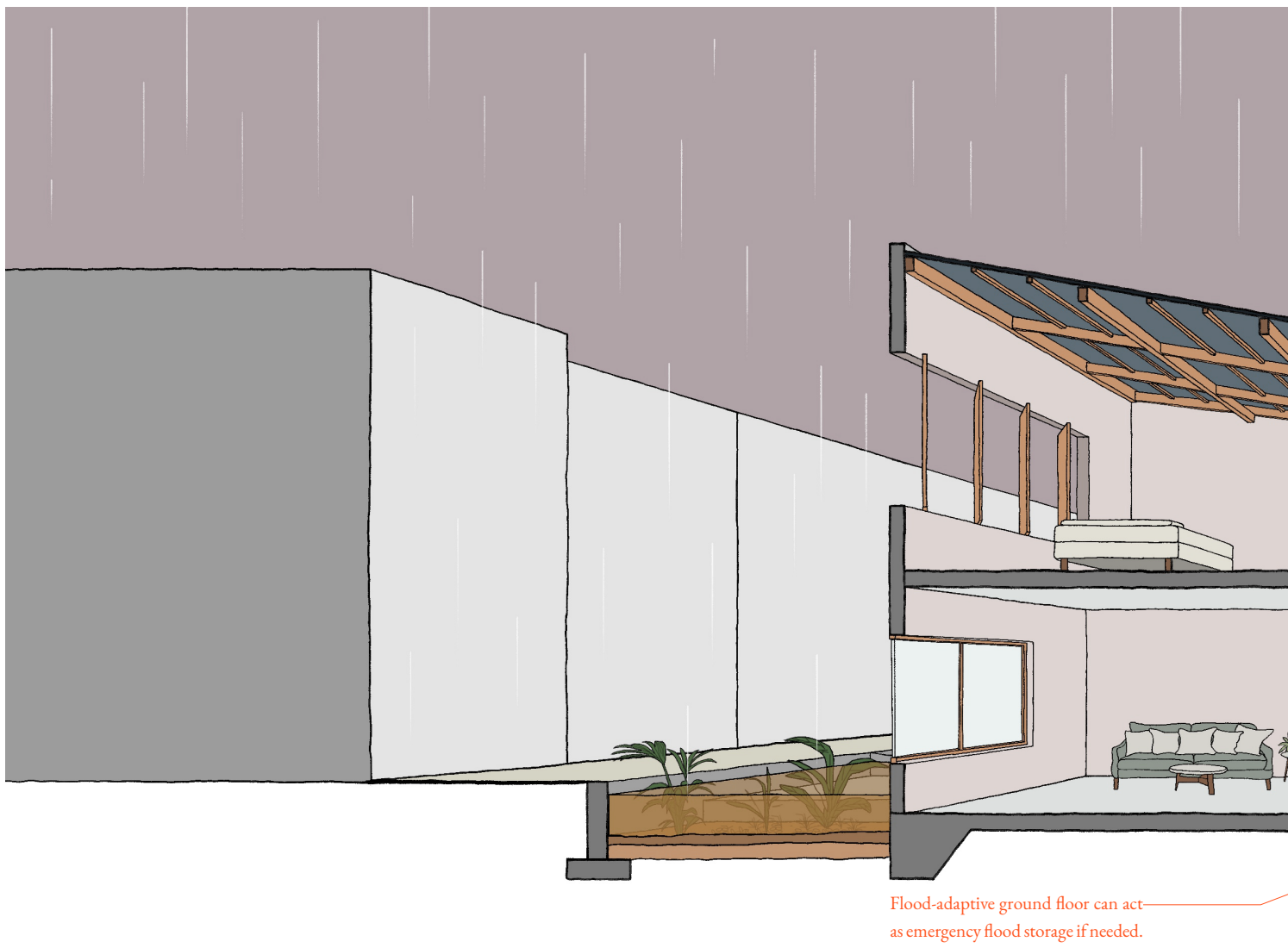
Fig. 4.24 Section of a new flood-adaptive alleyway house in flood condition
