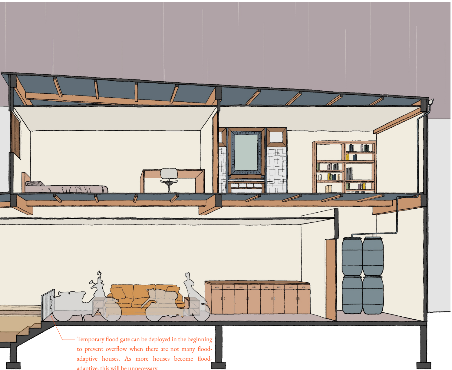
Fig. 4.14 Section of retrofitted alleyway house without front yard in flood condition.
