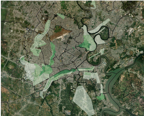
Fig. 0.12 This GIS map is an intersection of the official flood map and population statistic. It shows that at least 4,942,262 people (67%) affected by flooding. Different shades of green show different densities.
