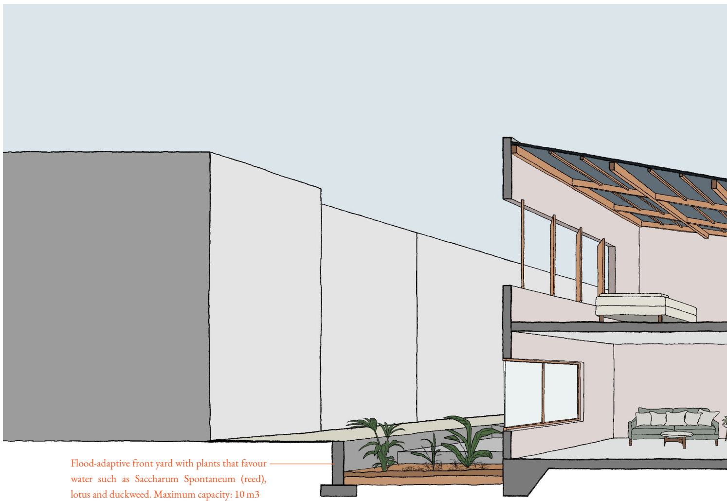
Fig. 4.22 Section of a new flood-adaptive alleyway house that is designed to accommodate a substantial amount of rainwater with flood-adaptive front yard and rainwater storage.
