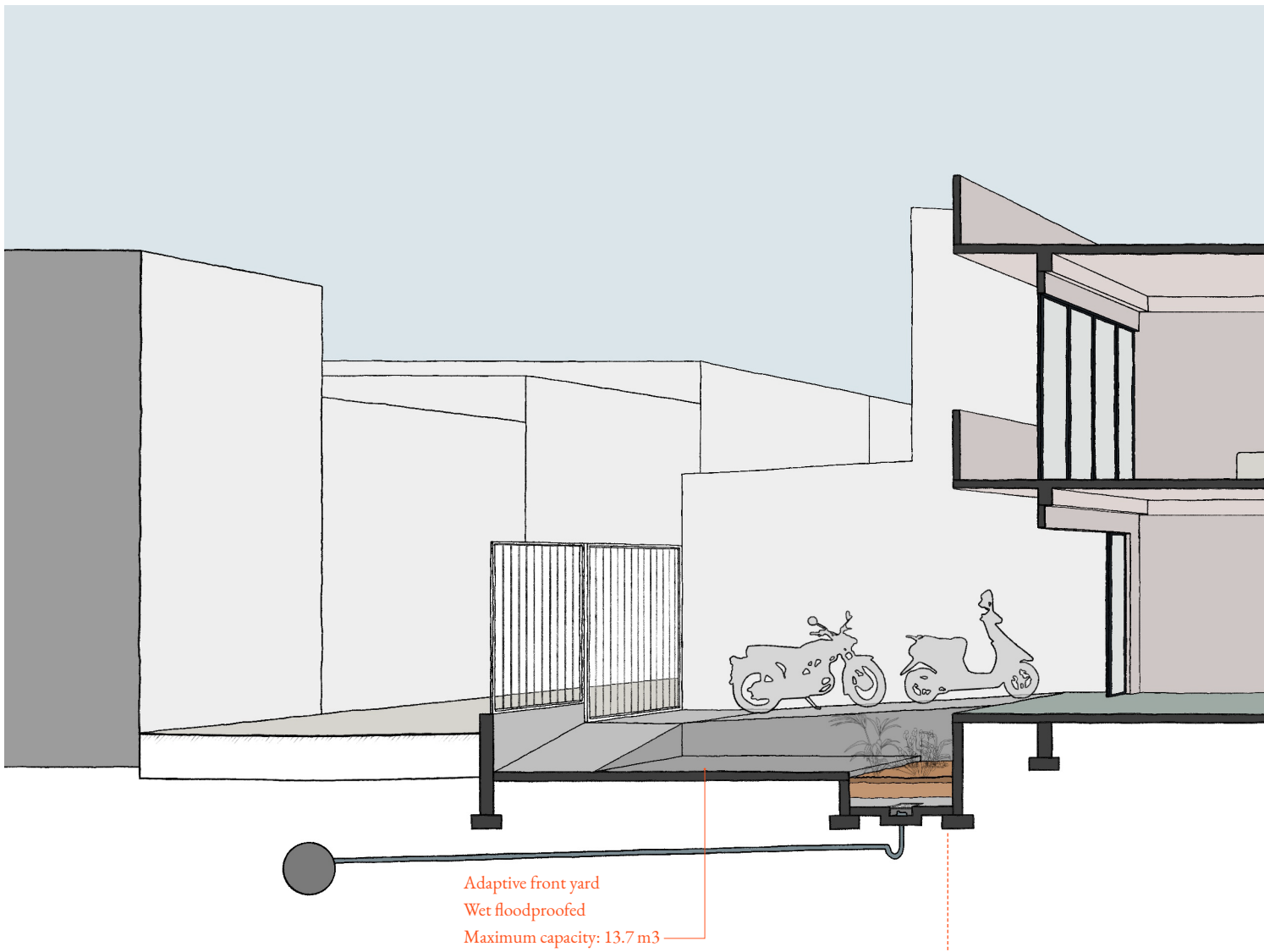
Fig. 4.16 Section of retrofitted alleyway house with front yard in dry condition.
