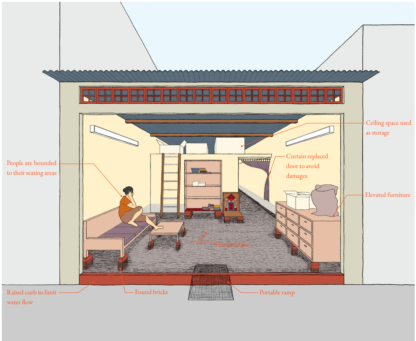
Fig. 2.25 One-point perspective showing how people temporarily adapt to flooding.
