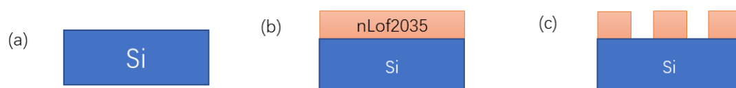
Fig. 4.1 Fabrication process of resist structure. (a) Bare Si wafer; (b) Spin-coat nLof2035 photoresist; (c) Exposure and development.
