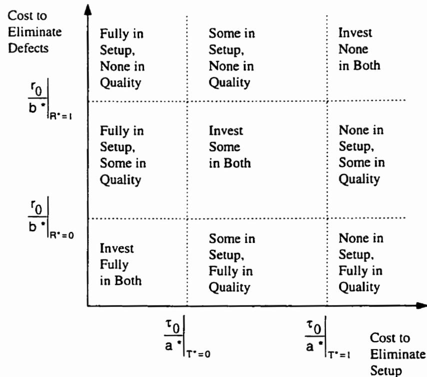
**Figure 3.5:** Schematic of Decision Matrix based on Costs to Eliminate Setup/Defects.
