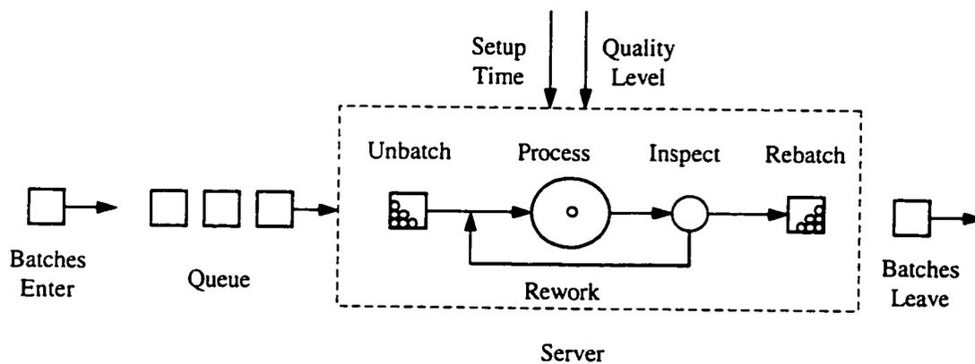
**Figure 3.2:** Detailed View of Physical System Model.
