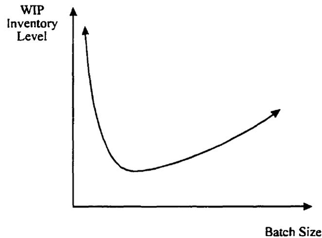
**Figure 2.2:** WIP Inventory as a function of Batch Size (following Karmarkar [1987])
