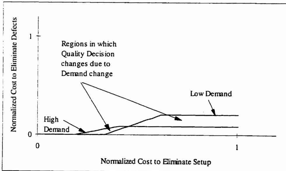
**Figure 4.17:** Decision Matrix for High and Low Defect Rates
