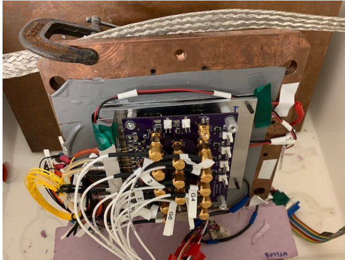
Figure 4.12: Final assembly of PCB, SPADs, TECs and copper heat sink, photographed during radiation testing experiment with appropriate readout and control cables.
