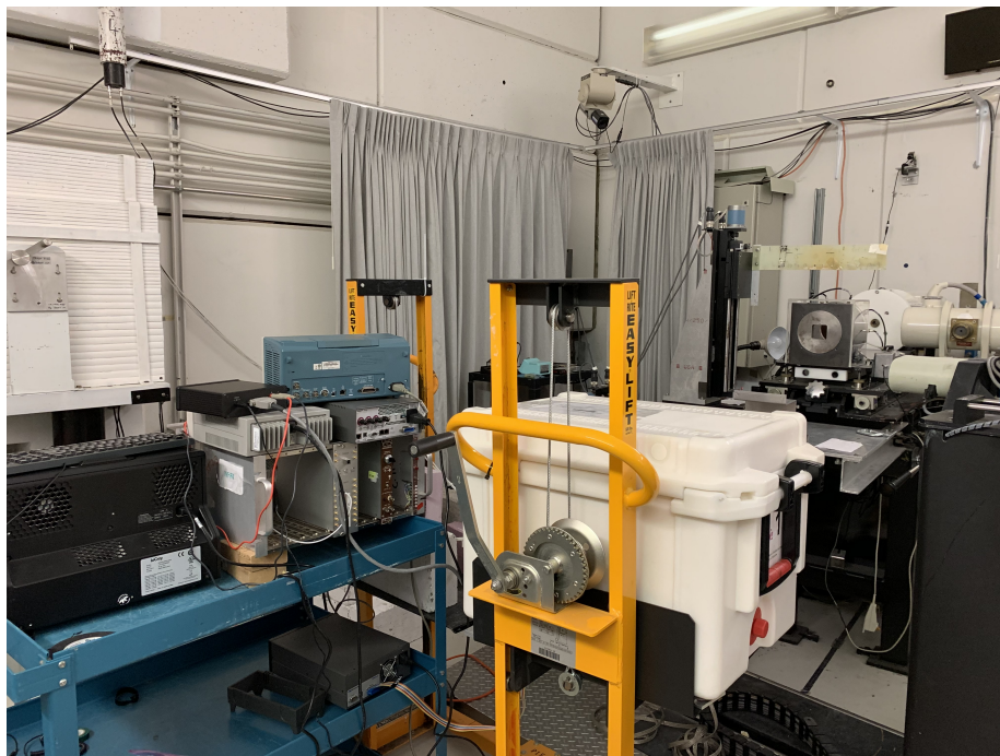
Figure A.9: Cooler containing detectors and electronics stands on height-adjustable platform. Proton beam port exit visible in the background. Oscilloscope, power supply and other control electronics were kept to the side of the radiation path.
