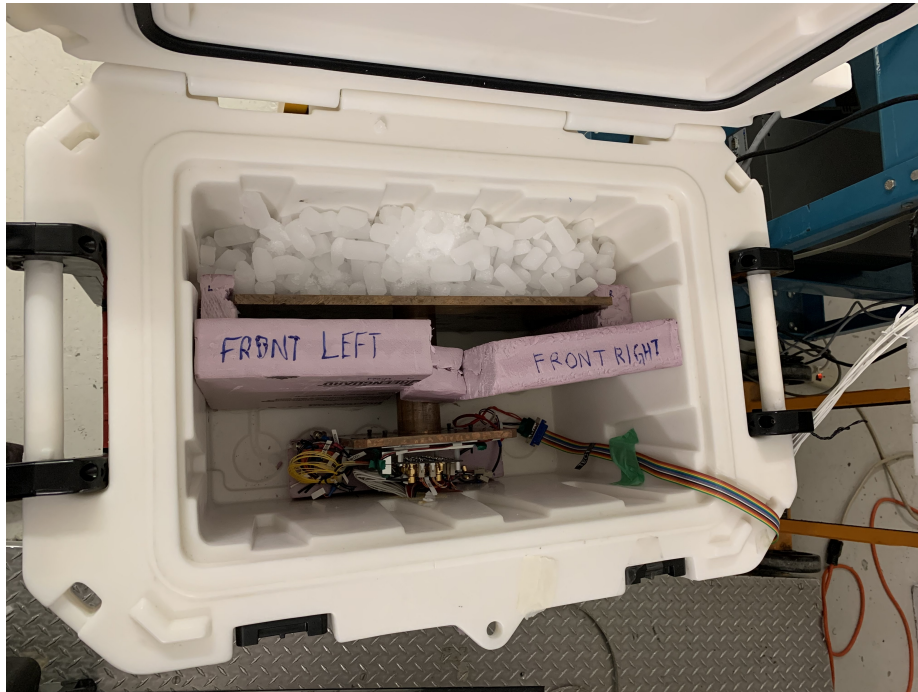
Figure A.11: Top view of detectors in cooler were dry ice pellets. TEC driver cable (rainbow flat cable) goes through crack between cooler and lid, while all other cables go through hole previously drilled in middle of cooler
