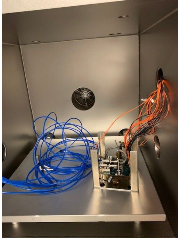
Figure 5.19: Photo of the CAPSat prototype DM inside the TVAC. The detectors are fiber coupled to the blue fibers which relay the optical annealing beam as well as a low-level light source used for characterization of the detector sensitivity. The orange and black wires extend from the CAPSat detectors module to the right of the TVAC where there is a DSUB connector to connect to the microcontroller and power supply outside of the TVAC.
