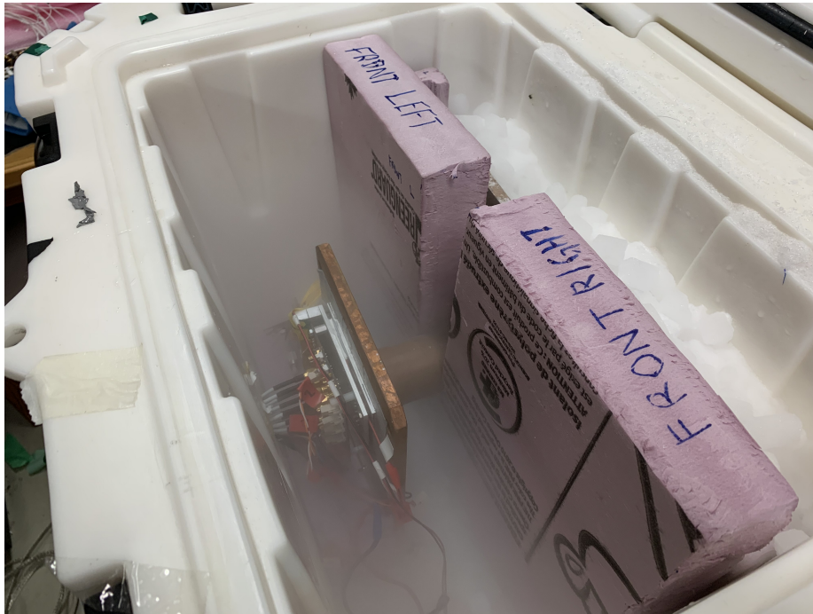
Figure A.14: Detector readout PCB mounted on copper heat sink abut to dry ice within the cooler. Foam was used to separate the ice from the front of the cooler where experimentalists work to make fine adjustments.
