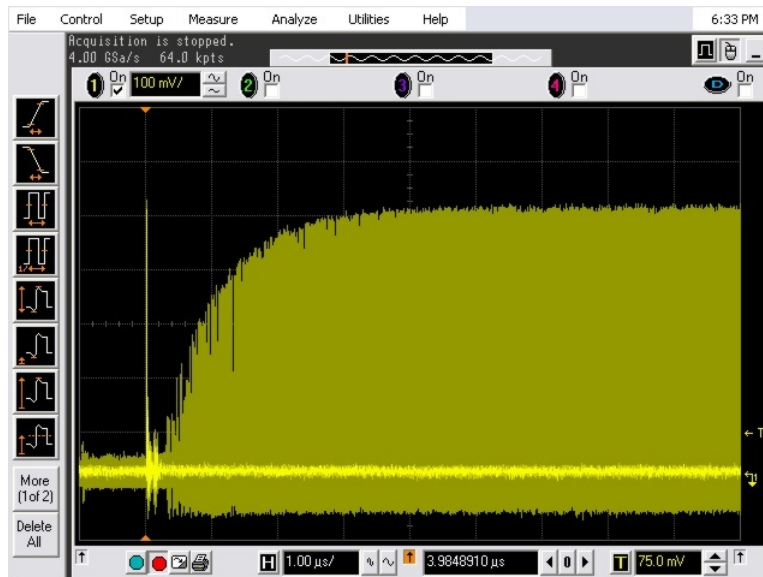
Figure 5.3: Oscilloscope screenshot of recharge time measurement.
