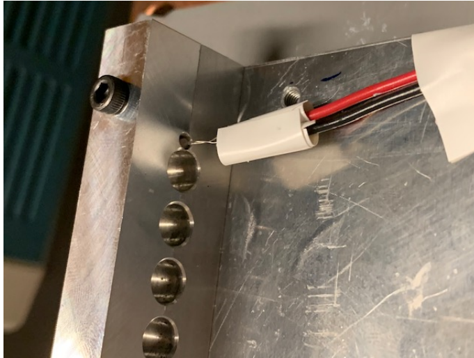
Figure 4.11: RTD temperature sensor in SPAD enclosure
