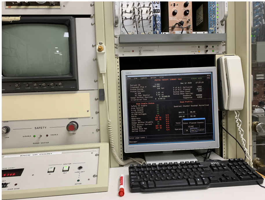
Figure A.16: Proton beam control room. Experimentalists called the cyclotron operator to provide the correct flux of protons, then used archaic computer system to set the exact dose needed. Before retirement, this system was used for radiation therapy of cancer patients.
