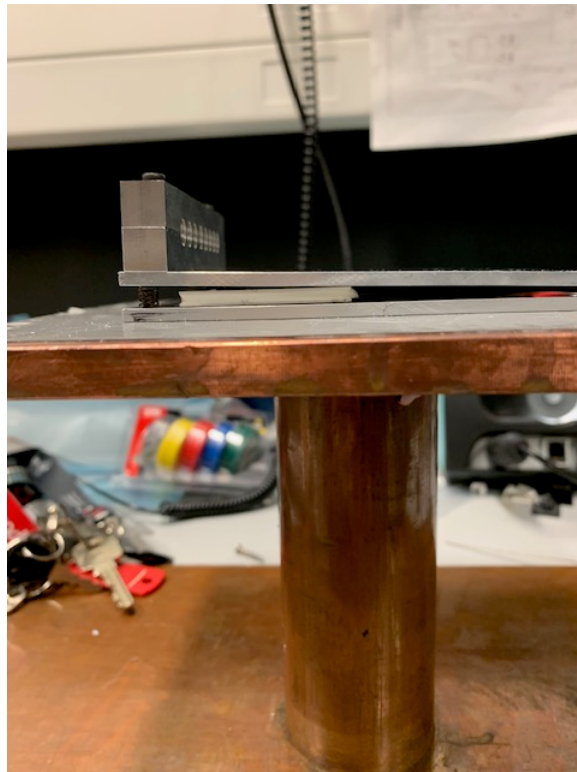
Figure 4.10: Side view of the TEC between aluminium plates on top of copper heat sink.
