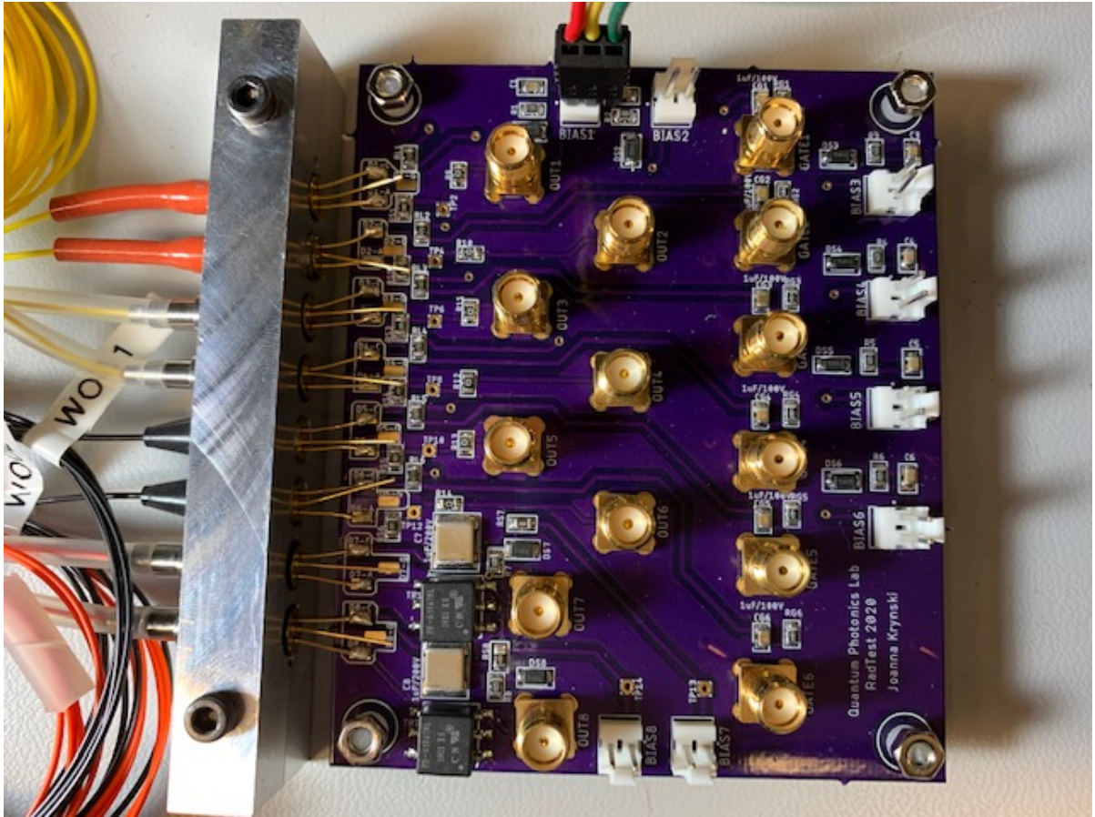
Figure 4.6: Final manufactured and populated PCB with attached SPADs in enclosure
