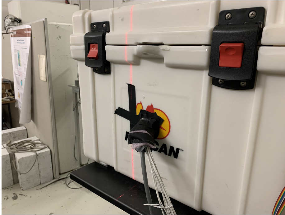
Figure A.12: Cooler cable hole stuffed with foam and tape to prevent leakage of cool air and moisture from entering the cooler. Power and signal cables are visible.
