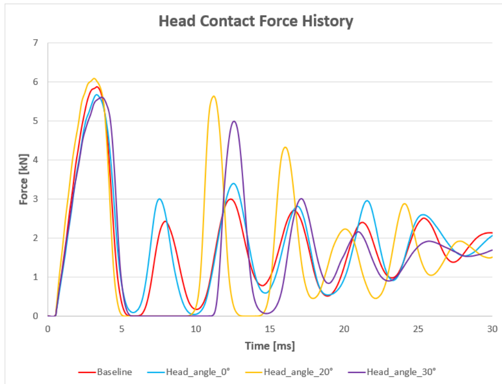
Figure 4-57: Head contact force history plots of baseline, Head_angle_0°, Head_angle_20°, and Head_angle_30° models
