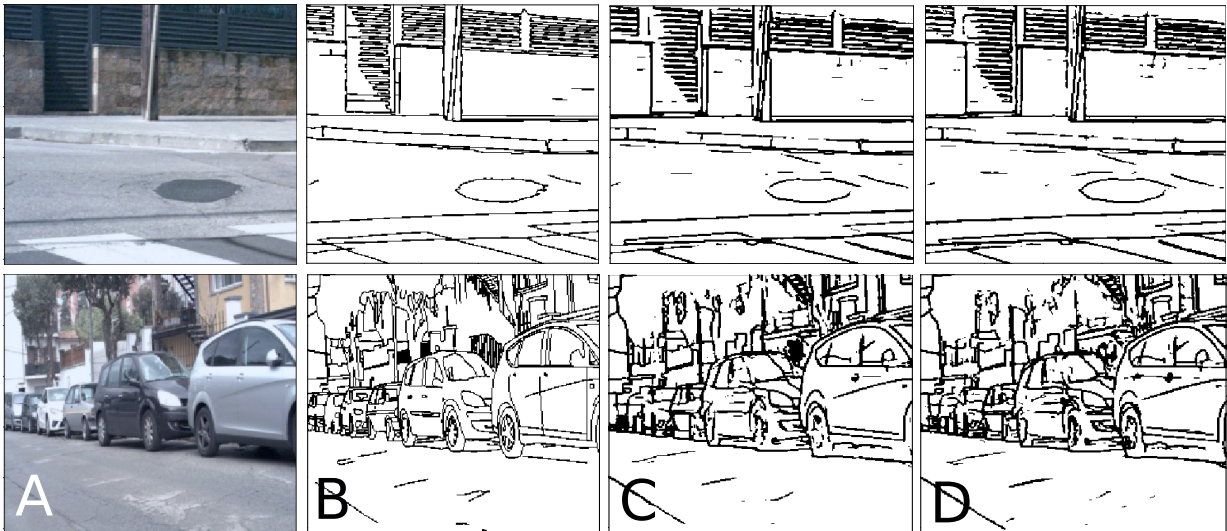
Figure 5.1: Edge detection in natural images stimuli. A, Example images from the BIPED [Poma et al., 2020] dataset. Each row show a different image. B, Ground truth edge maps for input images shown in column A. C and D, Corresponding predictions of the control and model, respectively.
