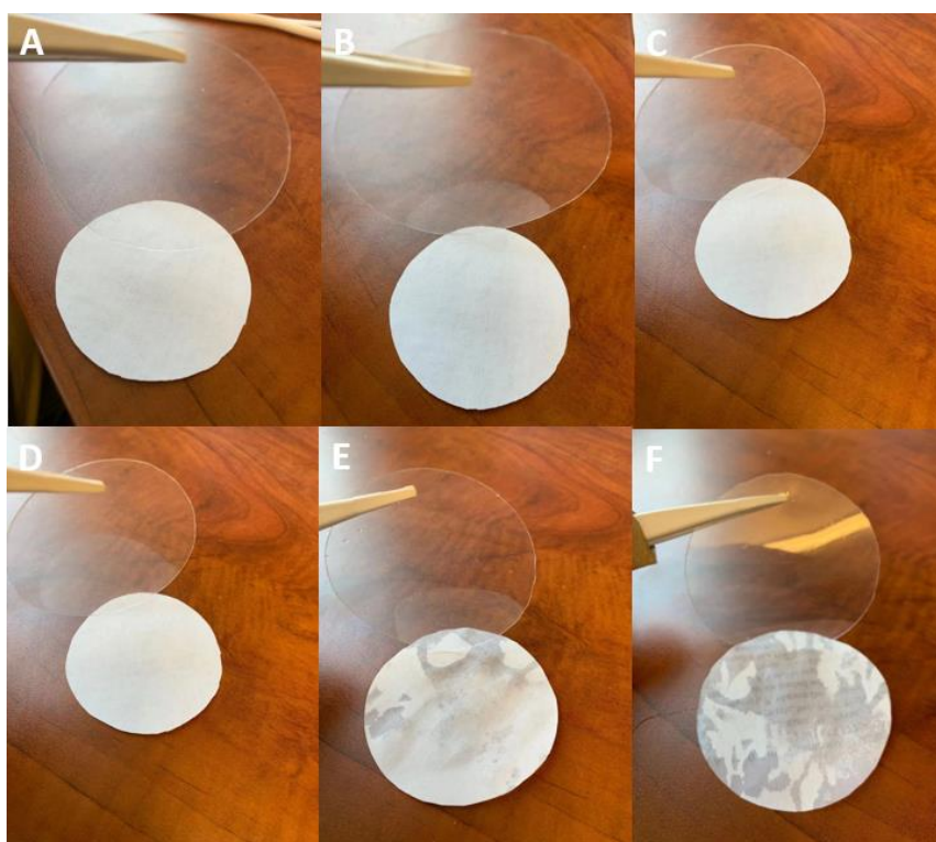
Figure 3.3 Image of transparent membranes: (A) PEBA, (B) 85PEBA/15DEHP, (C) 75PEBA/25DEHP, (D) 50PEBA/50DEHP, (E) 26PEBA/74DEHP and (F) 17PEBA/83DEHP.
